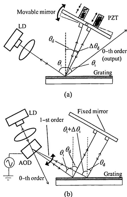
Fig. 1 Schematic of (a) conventional ECLD and (b) proposed system.
