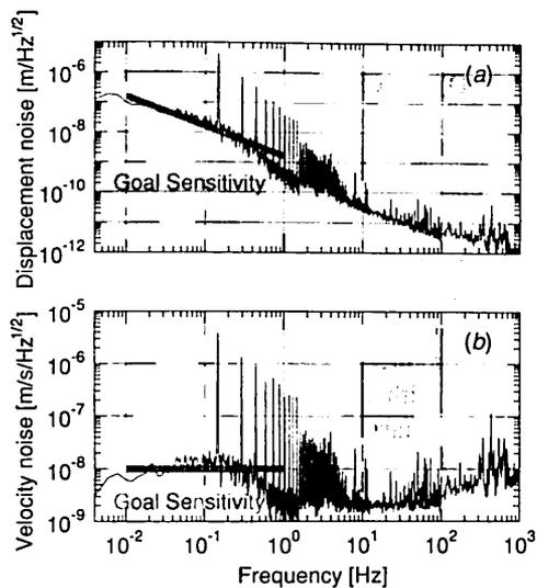
**Figure 6.** (a) Displacement noise spectrum and (b) velocity noise spectrum of Mach-Zehnder interferometer. The goal sensitivity of the SSI for a Japanese satellite gravity mission is also indicated by the grey lines.
