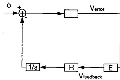
**Figure 3.** Block diagram of feedback control loop.  $I$  represents the frequency response for signal detection.  $E$  and  $H$  are the frequency response of a servo filter and that of a voltage–frequency converter, respectively.  $s$  denotes the Laplace frequency variable and  $\phi$  is the integration of Doppler frequency caused by mirror motion.
