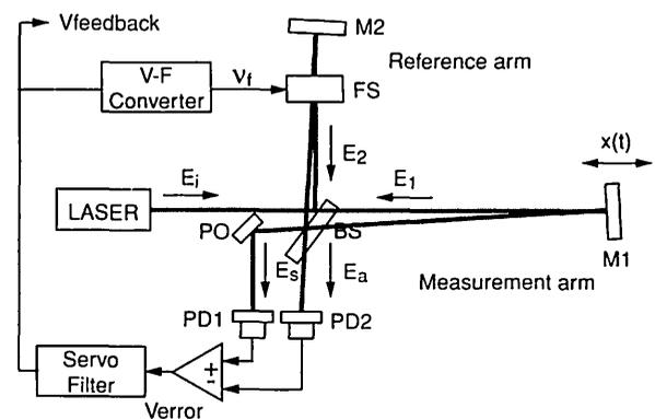
**Figure 2.** Conceptual design of a differential displacement measurement using an interferometer with a set of a frequency shifter and a voltage–frequency converter.  $E$ : light field,  $V$ : voltage,  $\nu_f$ : carrier frequency,  $x$ : displacement, BS: beamsplitter, M: mirror, PO: pick-off plate, PD: photodiode, FS: frequency-shifter and V–F converter: voltage–frequency converter.
