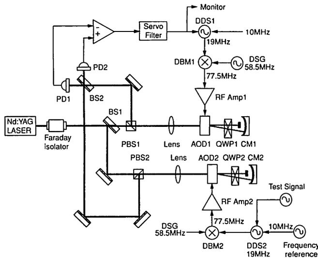
**Figure 4.** Schematic diagram of the Mach-Zehnder interferometer for differential displacement measurement. BS: beamsplitter, CM: concave mirror, QWP: quarter waveplate, PD: photodiode, AOD: acousto-optic deflector, DDS: direct digital synthesizer, DSG: digital signal generator and DBM: double-balanced mixer.
