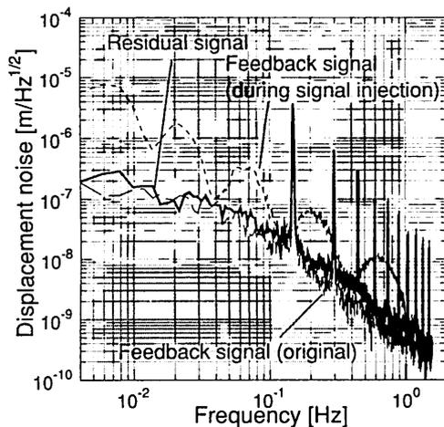
**Figure 7.** Residual spectrum of retrieved displacement signal. The solid and dotted lines are the residual spectrum and the feedback signal spectrum to the frequency shifter, respectively. The dashed line indicates the displacement noise spectrum of the Mach-Zehnder interferometer.
