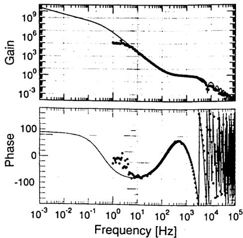
**Figure 5.** Measured open-loop transfer function of the feedback control system. The bold line and dots represent calculated and measured open-loop transfer functions of the feedback control loop, respectively.
