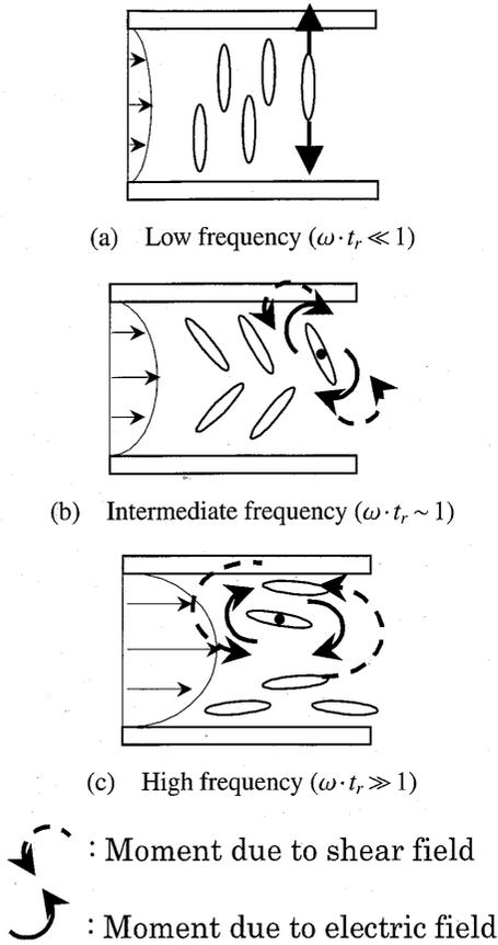
Fig. 6 Schematic images of molecular motion of liquid crystal subject to oscillatory shear flow and electric field
