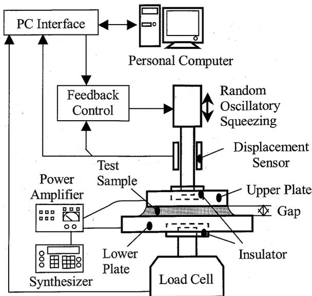
Fig. 2 Schema of experimental apparatus with Micro-Fourier Rheometer (MFR 2100)
