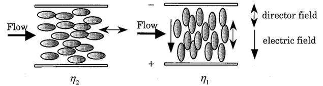
Fig. 1 Schematic mechanism of ER effect in liquid crystal ( $\Delta\epsilon > 0$ ). Note that the Miesowicz viscosities satisfy  $\eta_1 > \eta_2$
