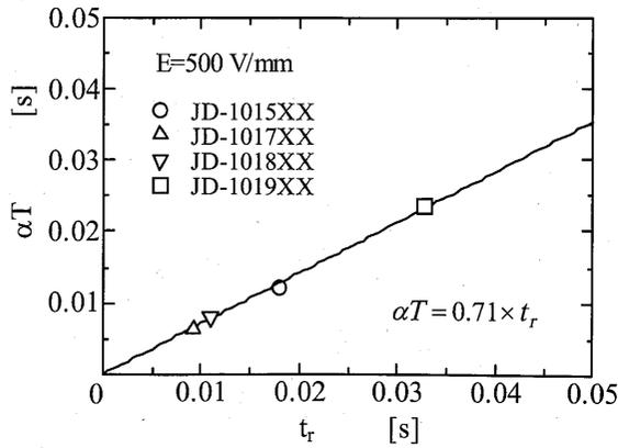
Fig. 8 Correlation between the two characteristic times,  $T$  and  $t_r$
