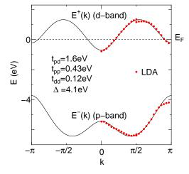
Fig. 2. A typical energy dispersion relation for the CuO double chain. Solid lines are the tight-binding result  $E^{\pm}(k)$  with  $t_{pd}=1.6 \mathrm{eV},\ t_{pp}=0.43 \mathrm{eV},\ t_{dd}=0.12 \mathrm{eV}$  and  $\Delta=4.1 \mathrm{eV}.$  Closed circles are the LDA result for Y124. <sup>36)</sup> Dotted line indicates the Fermi level with n=0.57.
