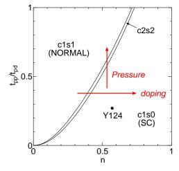
Fig. 3. Phase diagram on the n- $t_{pp}$  plane in the weak coupling limit for  $t_{pd}=1.6\mathrm{eV},~\Delta=4.1\mathrm{eV}$  and  $t_{dd}/t_{pp}=0.28$ . Closed circle stands for the parameter point corresponding to the LDA calculation for Y124.
