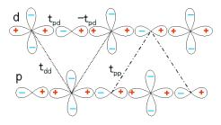
Fig. 1. Schematic diagram of  $\text{Cu}(3d_{x^2-y^2})$  orbitals and  $\text{O}(2p_\sigma)$  orbitals in a CuO double chain.
