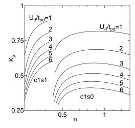
Fig. 4. The Luttinger parameter  $K_{\rho}$  as a function of the electron density n for several  $U_d$  for  $t_{pd}=1.6 \mathrm{eV},\ t_{pp}=0.43 \mathrm{eV},\ t_{dd}=0.12 \mathrm{eV}$  and  $\tilde{\Delta}=4.1 \mathrm{eV}.$
