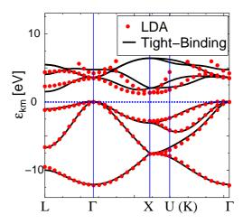
Fig. 1. The band structure for the Si crystal calculated from the  ${\rm LDA}^{24)}$  (closed circles) and from the tight-binding model (solid lines).
