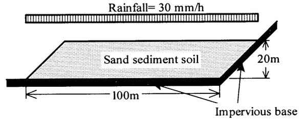
Figure 10: Numerical sand sediment soil to show practical influence of the gravel content on a prediction of storm runoff
