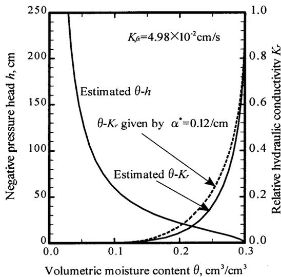
Figure 7: Unsaturated moisture properties of the sand estimated by the GA+FEM
