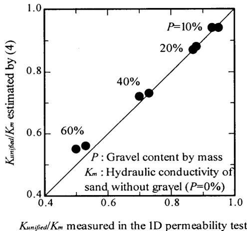
Figure 9: Comparison of the hydraulic conductivity of the sand-gravel mixture between the estimation by (4) and the laboratory permeability test
