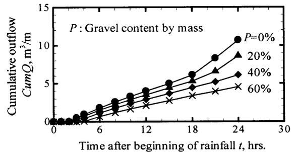
Figure 11: Cumulative outflow from the numerical sand sediment soil with time calculated by the FEM in which  $K_{unified}$  estimated by (4) is employed
