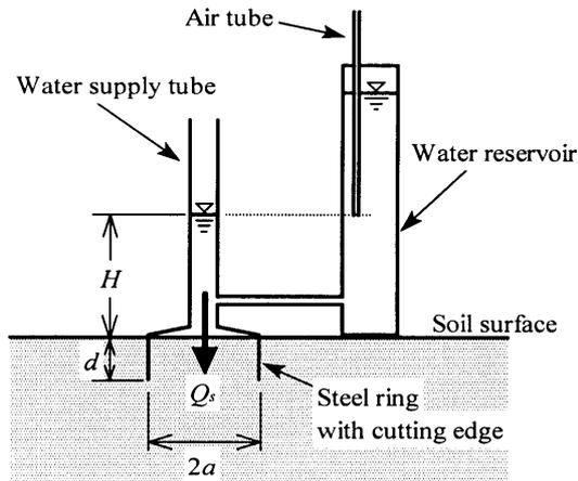
Figure 1: Schematic diagram of the GPI apparatus
