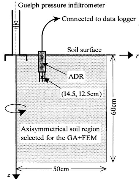
Figure 5: ADR inserted near the GPI ring to measure volumetric moisture content during infiltration
