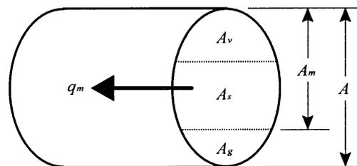
Figure 8: Descriptive cylindrical soil model assumed to derive the hydraulic conductivity of the sand sediment soil,  $K_{unified}$
