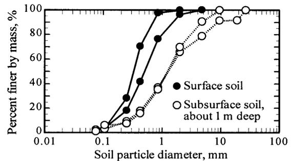
Figure 3: Grain size distribution of the sand tested
