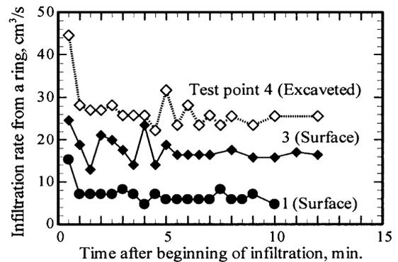
Figure 4: Typical examples of the infiltration rate measured during the in-situ permeability test using the GPI
