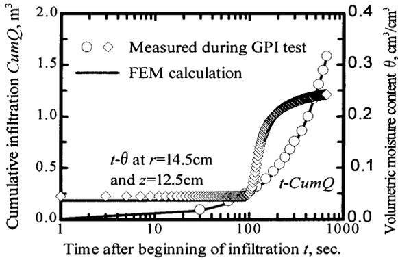
Figure 6: Comparison of cumulative infiltration and volumetric moisture content between the measurement and the FEM calculation after the GA+FEM iterations
