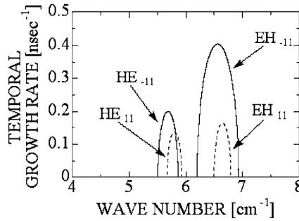
**Figure 2.** The temporal growth rates of nonaxisymmetric slow cyclotron instability with  $R_W = 1.445$  cm,  $R_d = 0.855$  cm,  $R_b = 0.8$  cm,  $\epsilon_r = 4$ ,  $B_0 = 0.8$  T,  $V_b = 660$  kV and  $I_b = 2.3$  kA.
