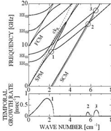
**Figure 1.** Dispersion curves of axisymmetric mode for the dielectric SWS system with  $R_W = 1.445$  cm,  $R_d = 0.855$  cm,  $R_b = 0.8$  cm,  $\epsilon_r = 4$ ,  $B_0 = 0.8$  T,  $V_b = 660$  kV and  $I_b = 2.3$  kA.
