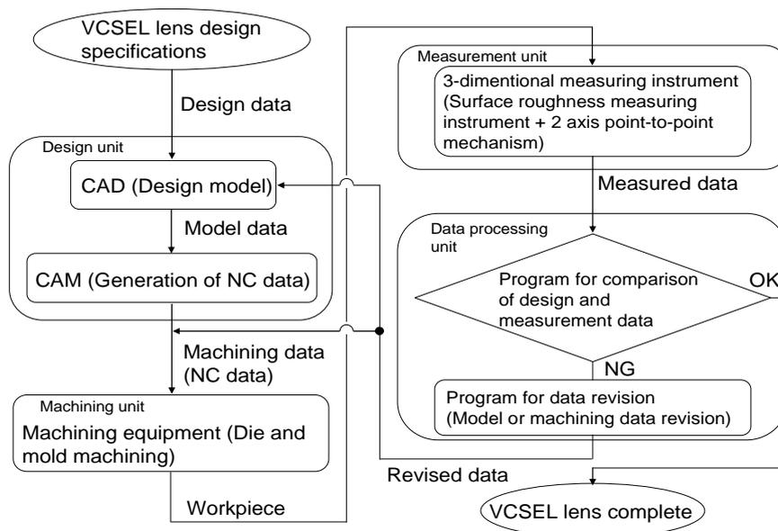
Fig. 1 Flow of online machining and measurement system.
