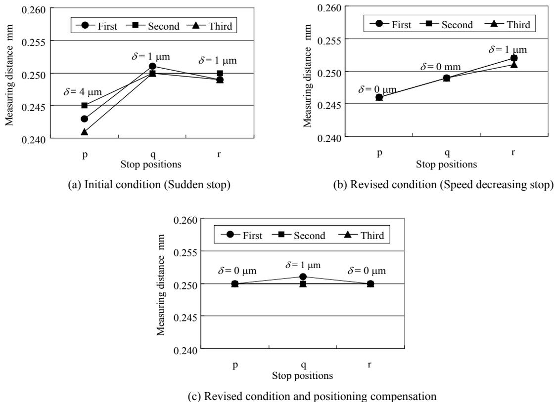
Fig. 2 Experimental results of performance of positioning instrument.
