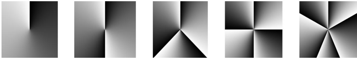
Fig.3.1 The hologram of phase mapping of vortex beam with the order of l=1,2,3,4 and 5 respectively.
