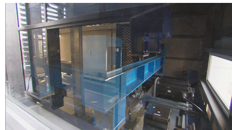
(b) Example of implementation of an active vibration absorber for a structure, the image cited from [7]
