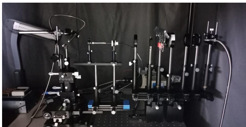
Figure 2.8 Picture of the SPR fluorescence spectroscopy instrumentation.
