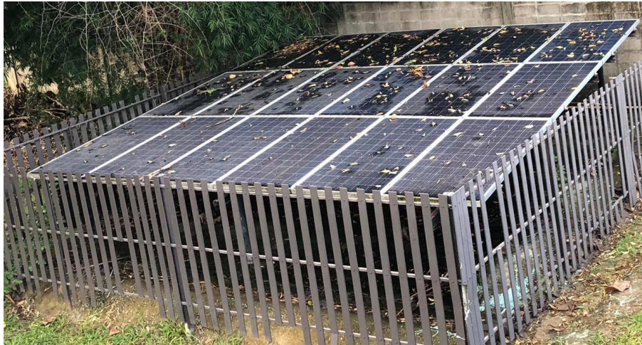
Figure 1.2. Monocrystalline silicon photovoltaic array.
