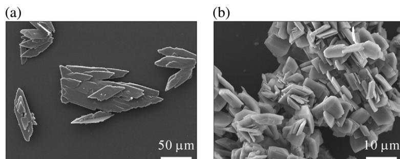
**Figure 2.** SEM micrographs of the products prepared via the solution method. (a) No additive, (b) with AE.
