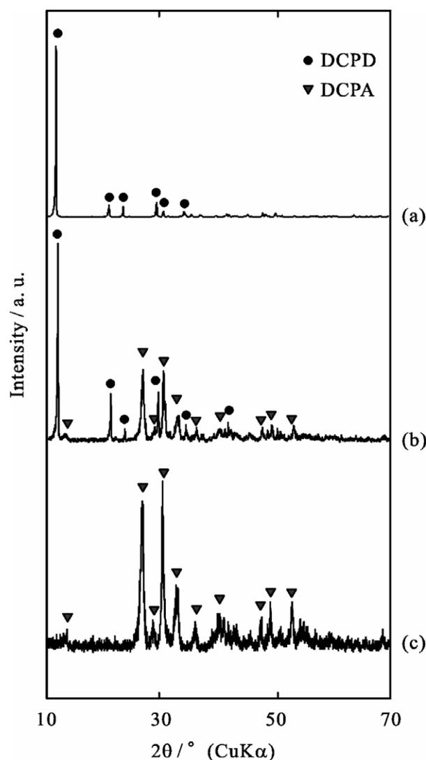
**Figure 3.** XRD patterns of the products prepared in the emulsion method at a Tween20 concentration of 0.5 wt% and Span80 concentrations of (a) 0.5, (b) 1, and (c) 5 wt%.
