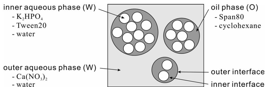
**Figure 1.** Construction of the multiple emulsion.
