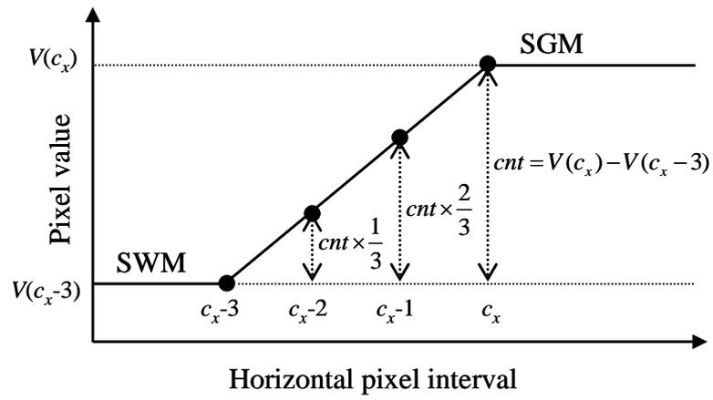
Fig.3 An explanatory diagram with regard to edge slope of SGM-SWM interface.
