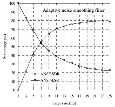
Fig.4 Graphs of SDR and ESR obtained from simulation images in condition of 400mAs, 6HU.
