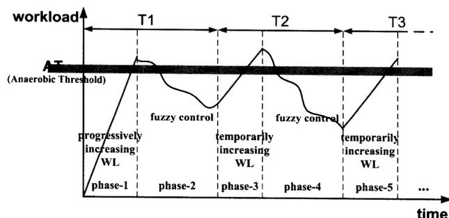
Fig. 2 A dynamic workload variation for cycle ergometer exercise.
