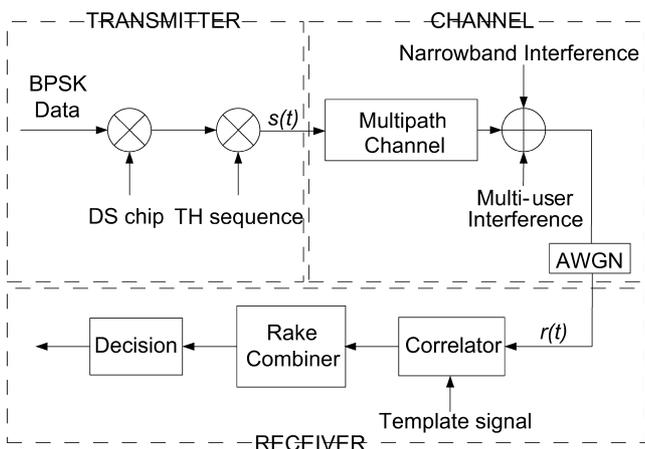
Fig. 1 Top diagram of UWB system.
