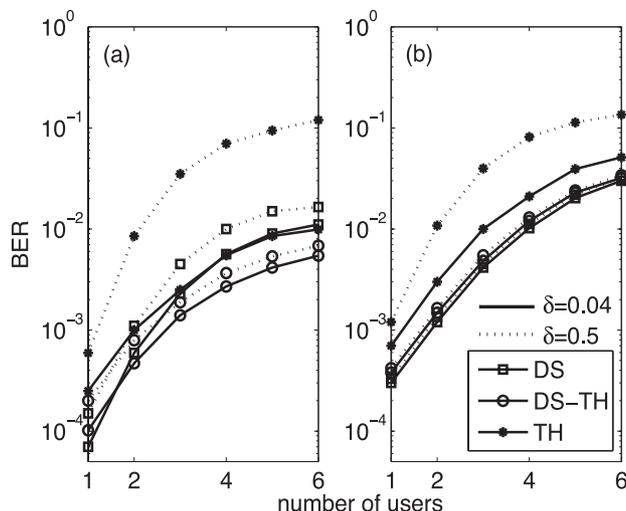
**Fig. 7** BER performance vs. number of users for DS, TH and DS-TH UWB systems. (a) CM1, (b) CM2. SNR=20 dB,  $L_c=8$ ,  $f_c=6$  GHz.
