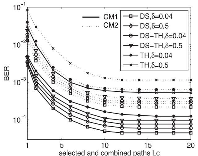
Fig. 5 BER performance vs. selected and combined paths  $L_c$  for DS, TH and DS-TH UWB systems. SNR=20 dB,  $W=2$  GHz,  $f_c=6$  GHz.
