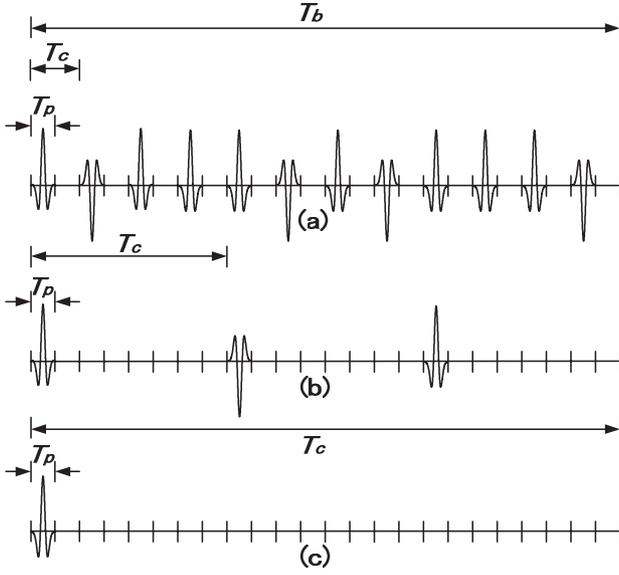
**Fig. 3** Illustration of signal with different pairs of DF and  $N_s$ , and with constant PG,  $W$  and  $R_b$ . (a)  $\delta=0.5$ ,  $N_s=12$ , (b)  $\delta=0.125$ ,  $N_s=3$ , (c)  $\delta=0.04$ ,  $N_s=1$ .
