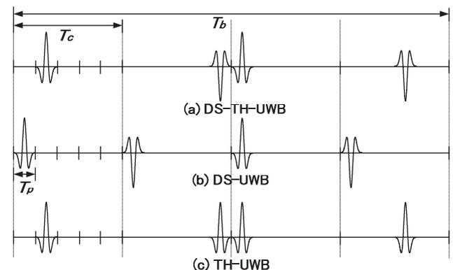
Fig. 2 Illustrations for (a) DS-TH-UWB, (b) DS-UWB and (c) TH-UWB signal. In this example,  $N_s=4$  and  $N_c=5$ .
