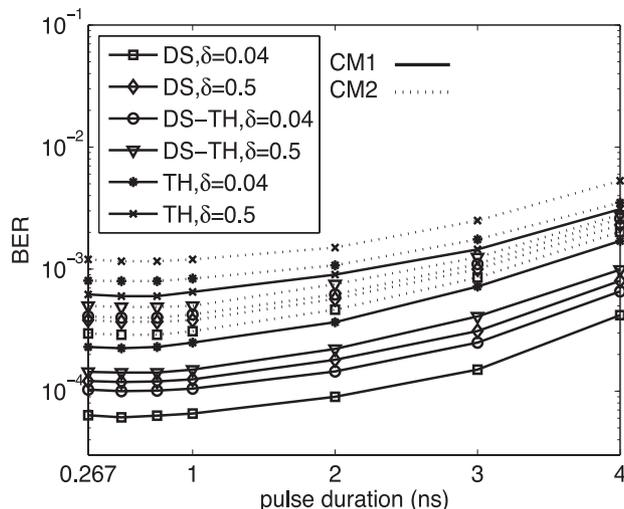
**Fig. 6** BER performance vs. pulse duration  $T_p$  for DS, TH and DS-TH UWB systems. SNR=20 dB,  $L_c=8$ ,  $f_c=6$  GHz.
