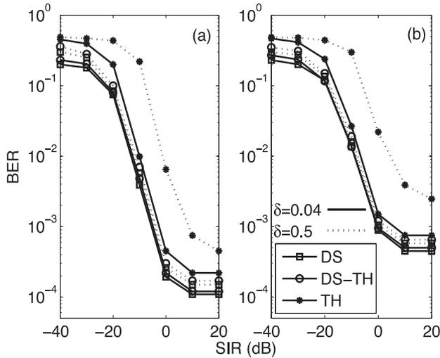
**Fig. 8** BER Performance vs. SIR for DS, TH and DS-TH UWB Systems. (a) CM1, (b) CM2. SNR=20 dB,  $L_c=8$ ,  $f_c=6$  GHz,  $f_{nrB}=6$  GHz,  $W_j=10$  MHz,  $U=1$ .
