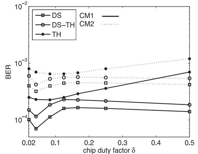
**Fig. 4** BER performance vs. chip duty factor for DS, TH and DS-TH UWB systems. SNR=20 dB,  $L_c=8$ ,  $W=2$  GHz,  $f_c=6$  GHz.
