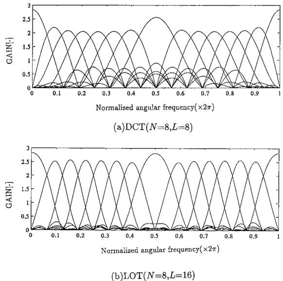
Fig. 3 Amplitude responses of analysis filter  $H_k(z)$ .
