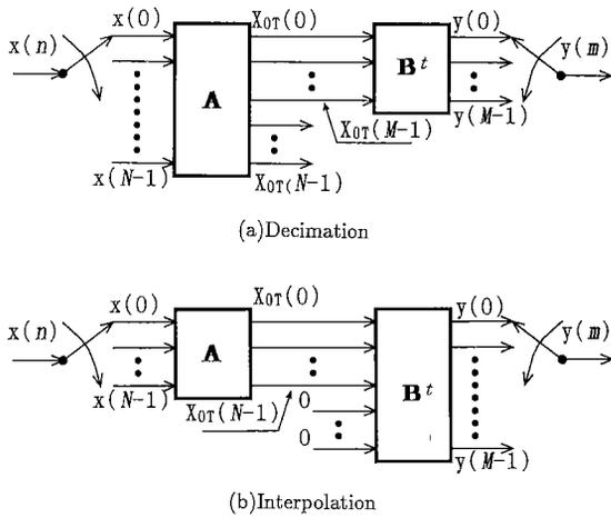
Fig. 1 Methods for conversion with orthogonal transform.
