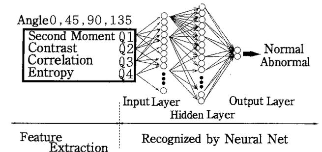
Fig. 4 Schematic diagram of the feature-based classification method using a neural network.
