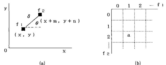
**Fig. 3** (a) Explanation of how to construct a gray-level cooccurrence matrix; (b) Layout of a gray-level cooccurrence matrix.
