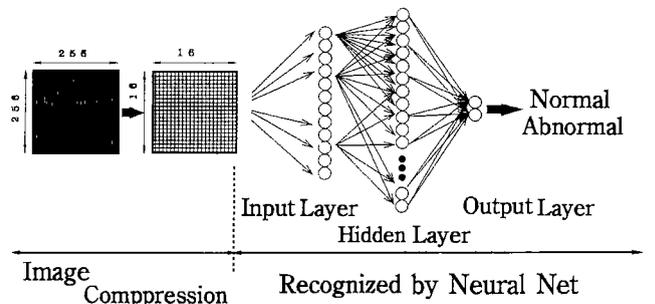
Fig. 5 Schematic diagram for image-based classification method using a neural network. The gray level of each pixel on the compressed image corresponds to an input unit.
