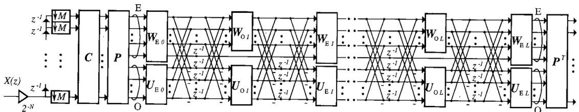
Fig. 2 Proposed lattice structure of  $M$ -channel LPPU analysis filter bank for an odd number of channel  $M$ .
