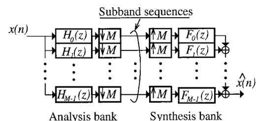
**Fig. 1**  $M$ -channel maximally decimated filter banks. The box including  $\downarrow M$  and  $\uparrow M$  denote the down- and up-sampler with the factor  $M$ , respectively.
