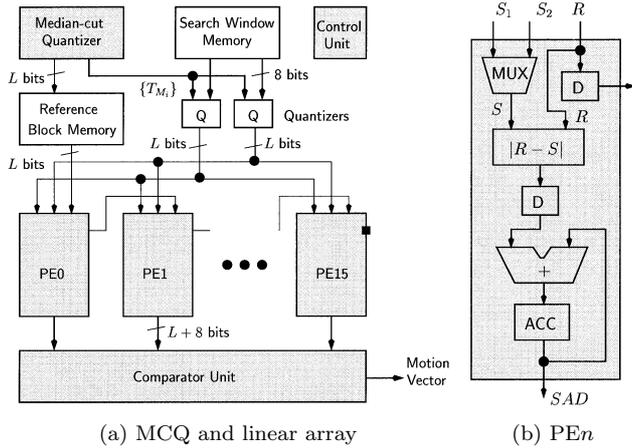
**Fig. 8** Linear array architecture of motion estimator with MCQ, where  $L$  denotes the number of quantized bits.
