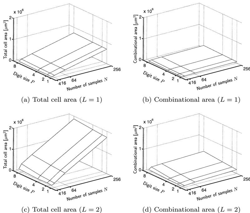
**Fig. 9** Cell area, which is estimated by Synopsis design compiler Ver.1998.02 from the VHDL model with the standard cell library EXDLIB provided by VDEC for  $0.5 \mu\text{m}$  triple-metal CMOS technology, where  $B = 8$ . CLK is constrained to  $80$  [nsec].
