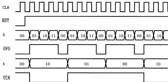
Fig. 7 Timing chart, where  $B = 3$ ,  $N = 8$  and  $P = 2$ .
