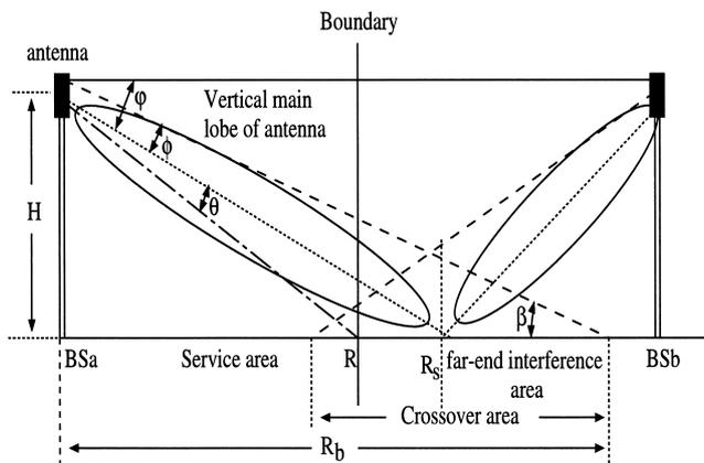
Fig. 3 Tilted antenna and shift of the boundary between cells.
