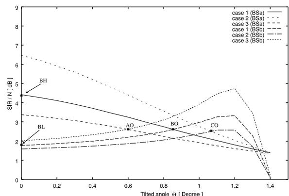
**Fig. 5**  $SIRs$  of  $BS_a$  and  $BS_b$  in the reverse link versus different tilted angle  $\theta$  ( $\frac{S_a}{S_b} = 1$ ,  $m = 0.5$ ,  $BW = 10$  degrees).
