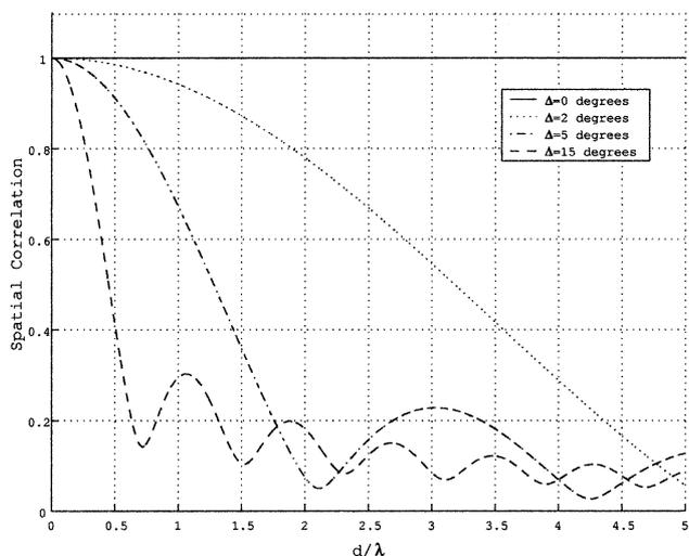
**Fig. 2** Spatial correlation versus  $d/\lambda$  with uniform distribution of angular energy ( $\phi=30$  degrees) for linear arrays shown in Fig. 1(a).
