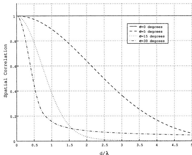
**Fig. 3** Spatial correlation versus  $d/\lambda$  with Gaussian distribution of angular energy ( $\phi=30$  degrees) for linear arrays shown in Fig. 1(a).
