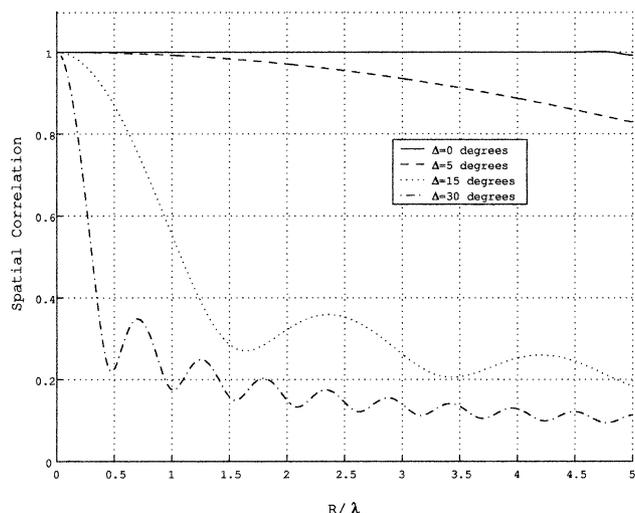
**Fig. 4** Spatial correlation between the elements 1 and 4 versus  $R/\lambda$  with uniform distribution of angular energy ( $\phi=30$  degrees) for circular arrays shown in Fig. 1(b).
