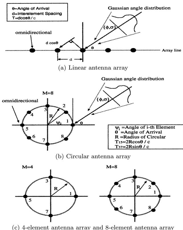
**Fig. 1** Signal angle determination in (a) linear antenna array and (b) circular antenna array, and (c) 4-element antenna array and 8-element antenna array.
