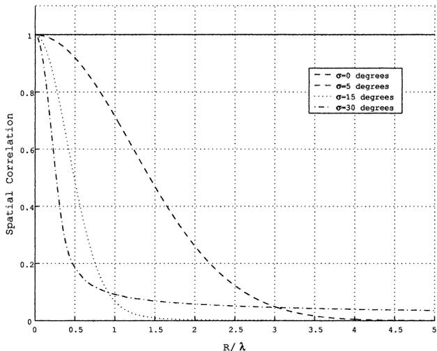
**Fig. 5** Spatial correlation between the elements 1 and 4 versus  $R/\lambda$  with Gaussian distribution of angular energy ( $\phi=30$  degrees) for circular arrays shown in Fig. 1(b).
