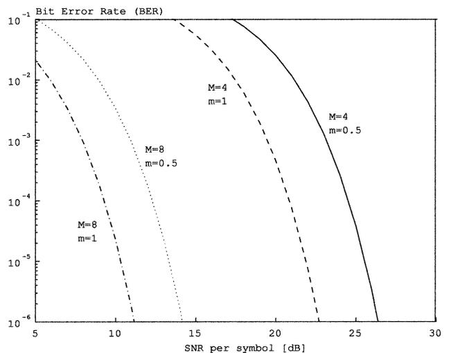
**Fig. 6** BER Performance versus SNR per symbol with Gaussian angle distribution for circular antenna arrays shown in Fig. 1(c) (DBPSK  $a=1$ ,  $R/\lambda = 1/4$ ,  $\sigma = 30$  degrees and  $\phi = 30$  degrees).
