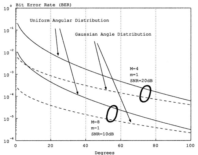
**Fig. 7** BER Performance versus  $\sigma$  and  $\Delta$  for circular antenna arrays shown in Fig. 1(c) (DBPSK  $a=1$ ,  $R/\lambda = 1/4$  and  $\phi = 30$  degrees).
