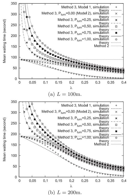
Fig. 8 Numerical results of  $E(T_{w,3})$  in Model 3 for  $P_{turn} = 0, 0.25, 0.5, 0.75$  and  $1.0$ , where  $n_c = 5$ .
