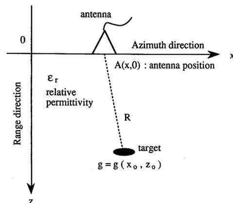
Fig. 2 Location of radar and target in a medium with  $\epsilon_r$ .
