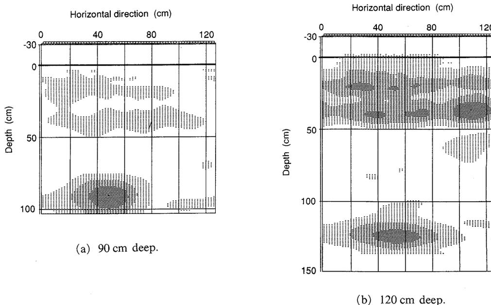
Fig. 8 Synthetic aperture image of a metallic plate (30 cm x 100 cm).
