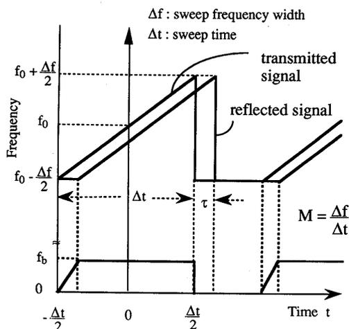
Fig. 1 Relation between frequency and time in FM-CW radar.
