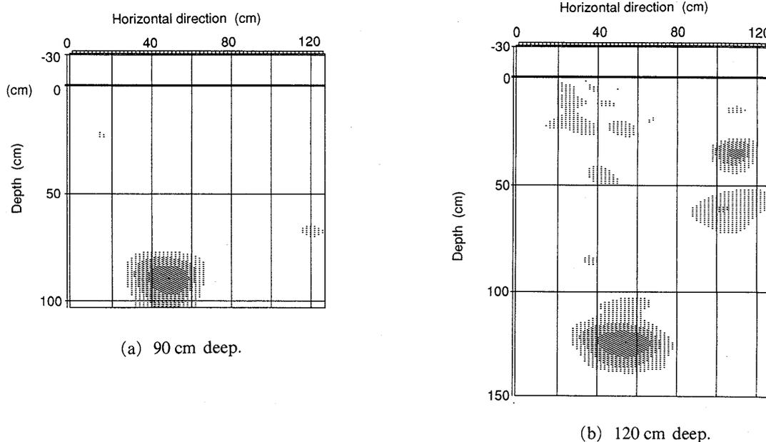
**Fig. 9** Processed image of a metallic plate by a method of averaging and subtracting.
