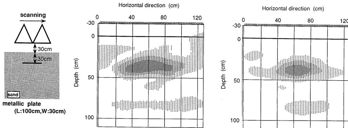
(a) Experimental scheme. (b) Real aperture image. (c) Synthetic aperture image.
