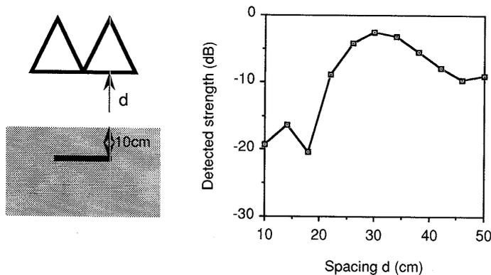
(a) Experimental scheme. (b) Detected strength.
