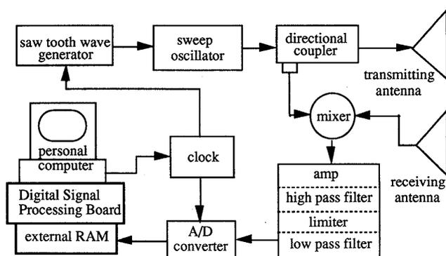
Fig. 4 Block diagram of FM-CW radar.
