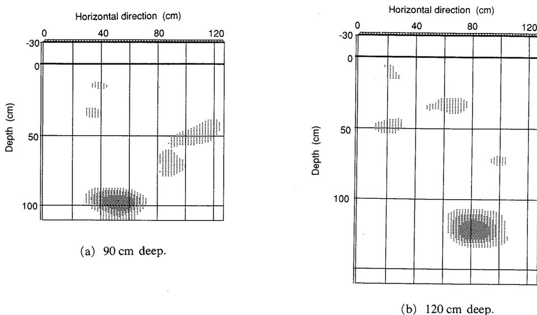
**Fig. 10** Processed image of a pipe (10 cm  $\phi$ ) by a method of averaging and subtracting.
