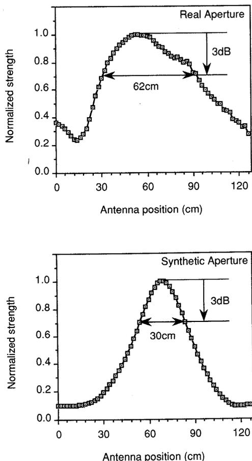
Fig. 7 Resolution by synthetic aperture processing.
