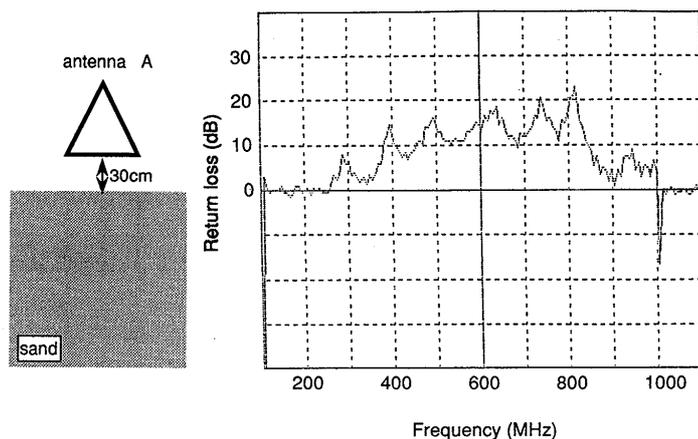
Fig. 3 Return loss of a ridged horn antenna.
