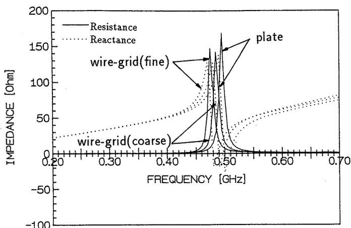
Fig. 8 Impedance vs. frequency for the antenna shown in Fig. 7.
