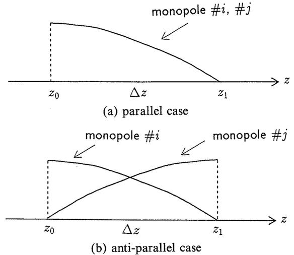
Fig. 2 A local coordinate system for calculating loss term of the additional mutual impedance between monopole  $\#i$  and  $\#j$ .
