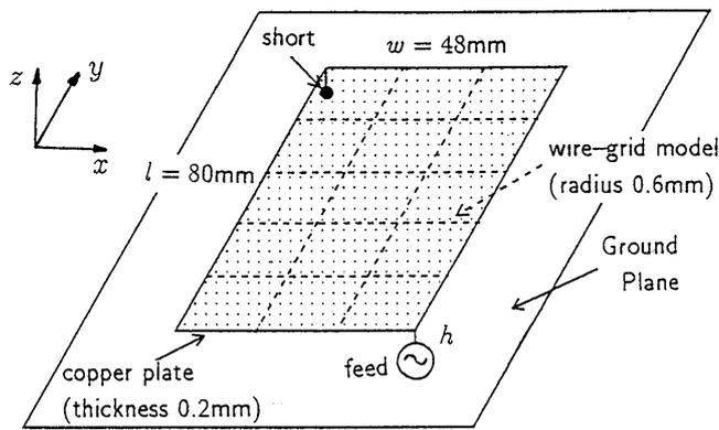
Fig. 1 A typical card-sized antenna for the paging.
