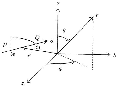
**Fig. 3** A coordinate system for calculating the far-field of a monopole.
