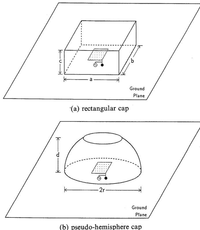
**Fig. 4** Shape of the shielding cap.
