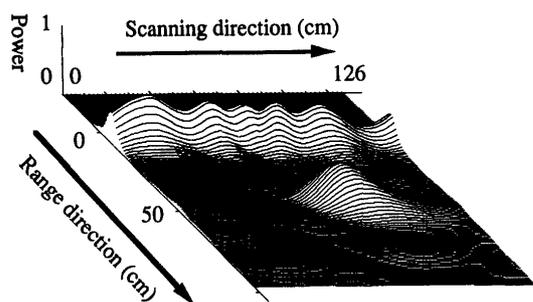
Fig. 4 Co-pol maximum image for the plate.
