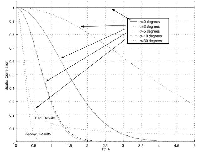
**Fig. 5** Spatial correlation between the elements 1 ( $\Psi_1=0$  degree) and 4 ( $\Psi_4=135$  degrees) versus  $R/\lambda$  with Gaussian distribution of angular energy ( $\phi=30$  degrees,  $\xi=90$  degrees) for circular array.
