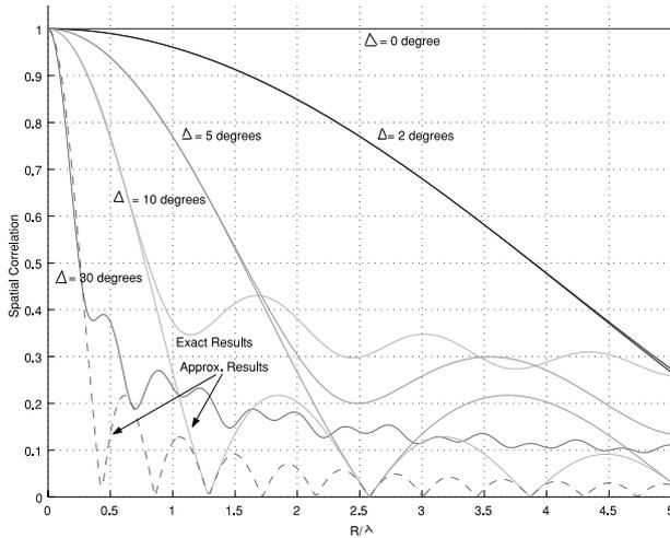
**Fig. 2** Spatial correlation between the elements 1 ( $\Psi_1=0$  degree) and 4 ( $\Psi_4=135$  degrees) versus  $R/\lambda$  with uniform distribution of angular energy ( $\phi=0$  degrees,  $\xi=90$  degrees) for circular array.
