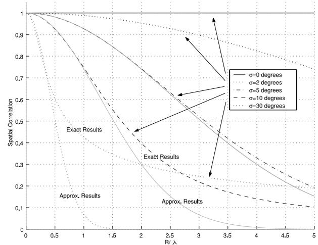
**Fig. 4** Spatial correlation between the elements 1 ( $\Psi_1=0$  degree) and 4 ( $\Psi_4=135$  degrees) versus  $R/\lambda$  with Gaussian distribution of angular energy ( $\phi=0$  degrees,  $\xi=90$  degrees) for circular array.
