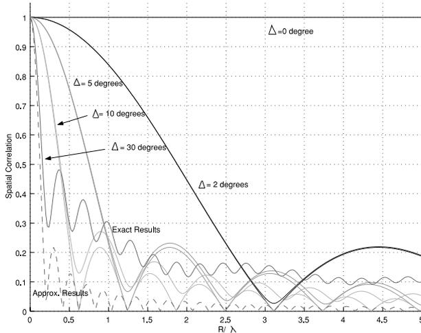
**Fig. 3** Spatial correlation between the elements 1 ( $\Psi_1=0$  degree) and 4 ( $\Psi_4=135$  degrees) versus  $R/\lambda$  with uniform distribution of angular energy ( $\phi=30$  degrees,  $\xi=90$  degrees) for circular array.
