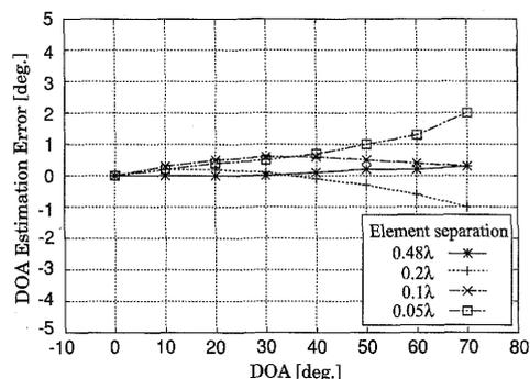
**Fig. 6** Estimated DOA errors with ULAs having various element separations.  $N = 4$ ,  $\theta_0 = 50^\circ$ ,  $\text{SNR} = \infty$  (no noise).
