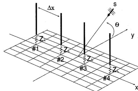
**Fig. 11** DOA estimation with 4-element monopole array.
