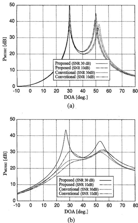
**Fig. 9** The MUSIC spectrum estimated by the finite SNR/snapshot data.  $N = 4$ ,  $\theta_1 = 30^\circ$ ,  $\theta_2 = 50^\circ$ , 50 snapshots. (a)  $0.48\lambda$  element separation, (b)  $0.48\lambda$  element separation.
