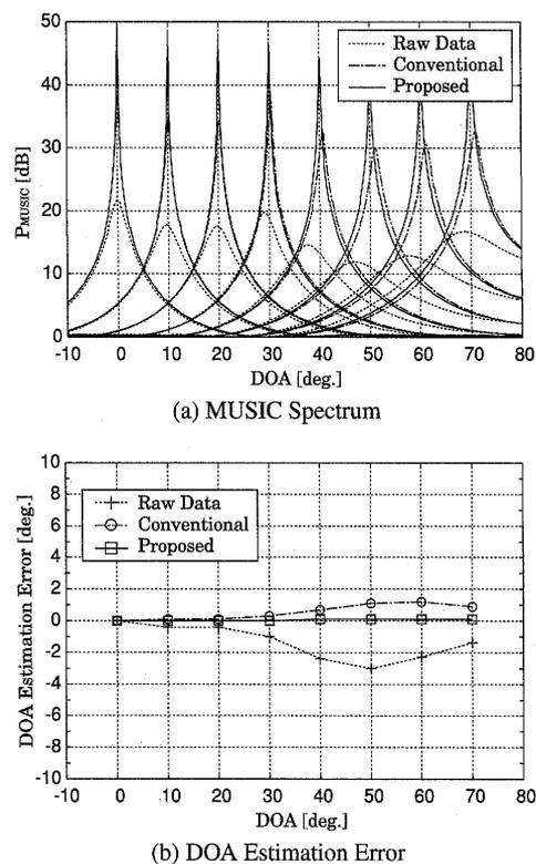
Fig. 3 DOA estimation results and estimation errors by the MUSIC algorithm.  $N = 4, \Delta x_{12} = \Delta x_{23} = \Delta x_{34} = 0.48\lambda, \text{SNR} = \infty$  (no noise).
