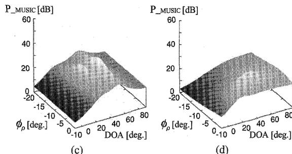
**Fig. 8** DOA and compensation coefficient estimation by the  $P_{MUSIC}(\theta, \phi_\rho)$  with finite SNR/snapshots.  $N = 4$ ,  $\theta_1 = 30^\circ$ ,  $\theta_2 = 50^\circ$ , 50 snapshots. (a)  $\text{SNR}=30$  dB,  $0.48\lambda$  element separation, (b)  $\text{SNR}=10$  dB,  $0.48\lambda$  element separation, (c)  $\text{SNR}=10$  dB,  $0.2\lambda$  element separation, (d)  $\text{SNR}=10$  dB,  $0.1\lambda$  element separation.
