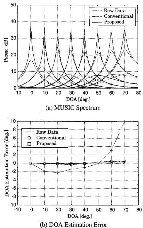
**Fig. 10** DOA estimation results and estimation errors by the MUSIC algorithm.  $N = 4$ ,  $\Delta x_{12} = \Delta x_{34} = 0.65\lambda$ ,  $\Delta x_{23} = 0.2\lambda$ ,  $\text{SNR} = \infty$  (no noise).
