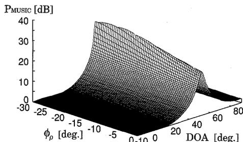
**Fig. 12** DOA and compensation coefficient estimation by  $P_{\text{MUSIC}}(\theta, \phi_\rho)$ .  $N = 4$ ,  $\Delta x = 0.498\lambda$ ,  $\theta_0 = 50^\circ$ , 1 snapshot.
