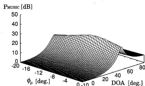
Fig. 4 The DOA and compensation coefficient estimation by  $P_{\text{MUSIC}}(\theta, \phi_\rho)$ .  $N = 4, \Delta x_{12} = \Delta x_{23} = \Delta x_{34} = 0.2\lambda, \theta_0 = 50^\circ, \text{SNR} = \infty$  (no noise).
