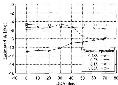
**Fig. 7** Estimated  $\phi_\rho$  with ULAs of various DOAs and element separations.  $N = 4$ ,  $\text{SNR} = \infty$  (no noise).
