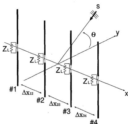
Fig. 1 DOA estimation with an  $N$ -element dipole array.
