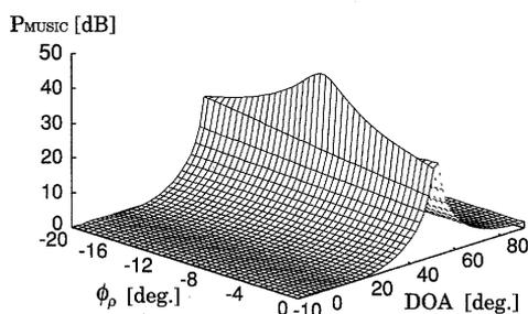
Fig. 2 The DOA and compensation coefficient estimation by  $P_{\text{MUSIC}}(\theta, \phi_\rho)$ .  $N = 4, \Delta x_{12} = \Delta x_{23} = \Delta x_{34} = 0.48\lambda, \theta_0 = 50^\circ, \text{SNR} = \infty$  (no noise).
