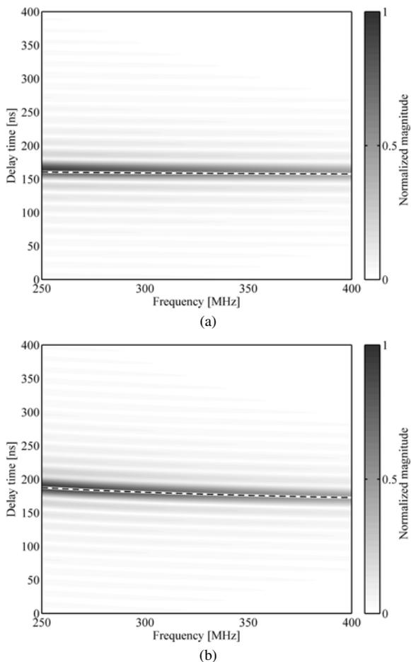
Fig. 7 Simulation results of observation frequency versus delay time of targets: (a)  $(z_T, r_T) = (20, 1)$ , (b)  $(20, 5)$  [m].
