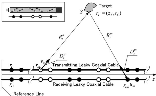
Fig. 4 Analysis model for target response.
