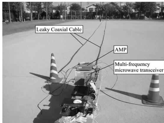
Fig. 9 Validation system of two-dimensional target location by leaky coaxial cables.
