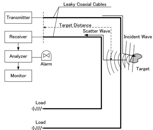
**Fig. 1** Basic configuration of the system and intrusion detection applications for leaky coaxial cables.
