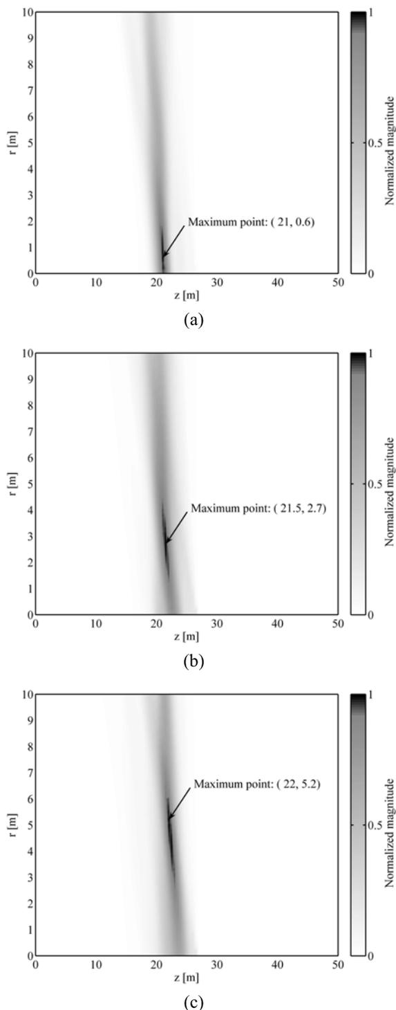
**Fig. 14** Reconstruction image based on Hough transform of target: (a)  $(z_T, r_T) = (20, 1)$ , (b)  $(20, 3)$ , and (c)  $(20, 5)$  [m].
