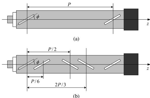
**Fig. 2** Configuration of leaky coaxial cables: (a) basic configuration; (b) wide bandwidth configuration with subslot.
