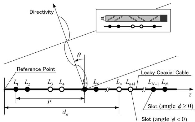
**Fig. 3** Slot array model of leaky coaxial cable.
