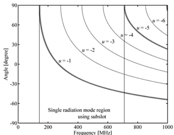
Fig. 6 Computation results of directivity of leaky coaxial cables.
