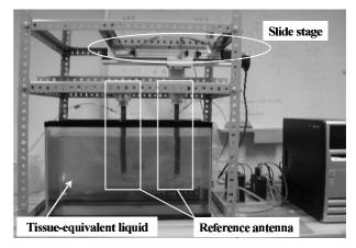
**Fig. 2** Measurement setup. Two reference antennas in the tissueequivalent liquid are connected to the slide stage so as to control their separation.
