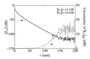
Fig. 4 Measured  $|S_{21}|_{dB}$  and corresponding uncertainty at 2.45 GHz.
