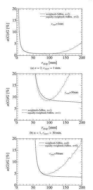
**Fig. 5** Variation in estimated far-field gain as a function of upper limit of the fitting range,  $r_{stop}$ .
