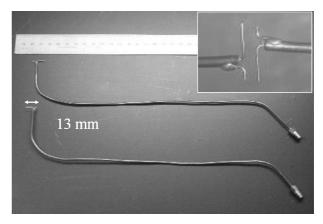
Fig. 3 Offset-fed dipole antennas and semi-rigid cables.
