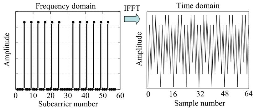
(a) Waveform of short preamble in IEEE802.11 based OFDM signal.
