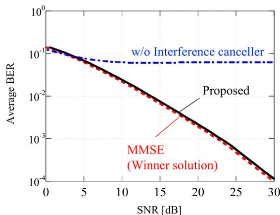
(b) Bit error rate versus SNR
