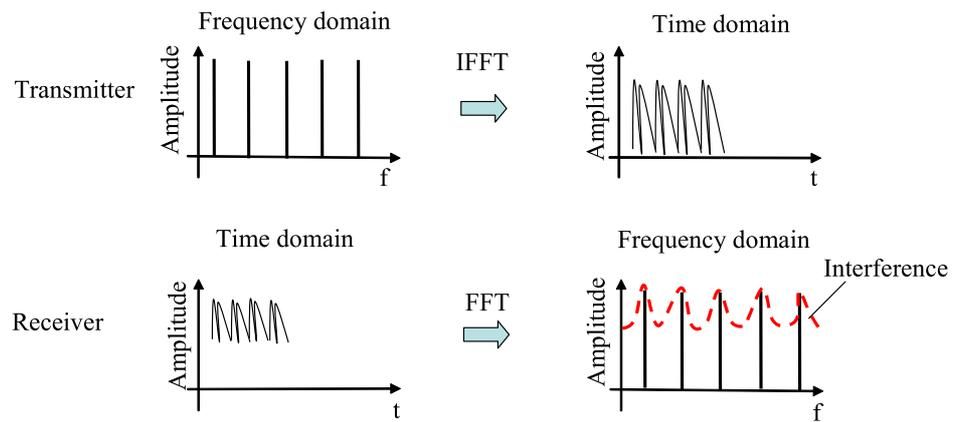
(b) Relationship between desired signal and interference in short preamble.
