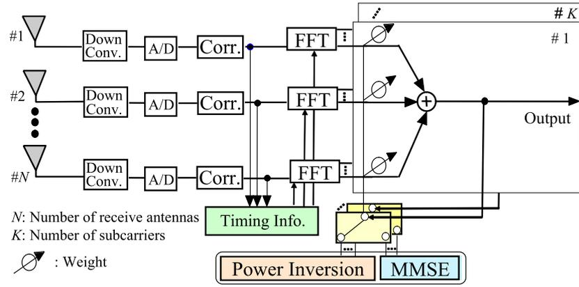
Fig. 2. Configuration of receiver by proposed method.
