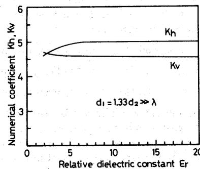
Fig. 10. Numerical coefficient versus relative dielectric constant.
