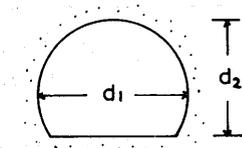
Fig. 8. Tunnel dimensions: width  $d_1$ , height  $d_2$ .
