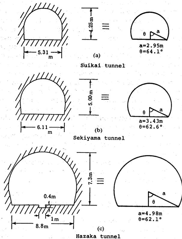
Fig. 4. The tunnel dimensions under measurement and equivalent dimensions of arched tunnels considered here.
