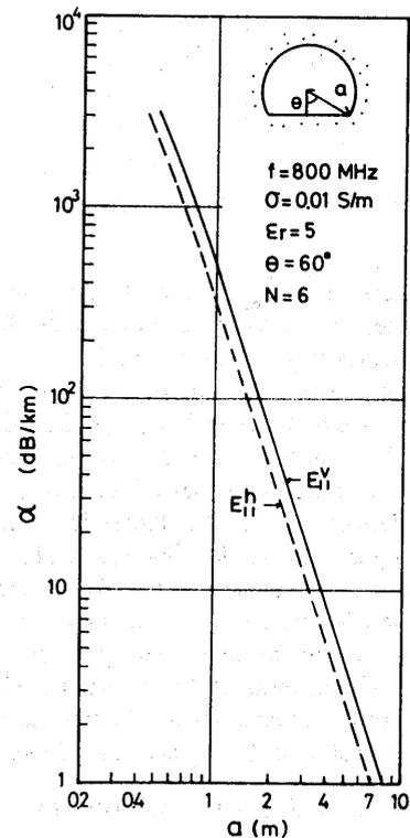
Fig. 6. Attenuation constant as a function of radius  $a$ .
