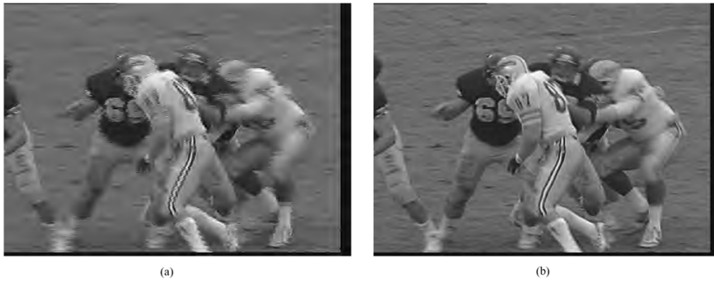
Fig. 13. Simulation results with the gain compensation decoded at 0.25 bpp. (a) \theta = 1.0 (field interleaving). (b) \theta = 0.25 .
