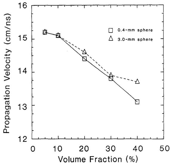
Fig. 3. Propagation velocity as a function of sphere volume fraction. Each marker represents the average velocity obtained from five different samples.
