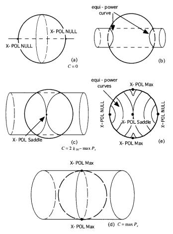
Fig. 3. Equi-power curves and the characteristic polarization states in the cross-pol channel.
