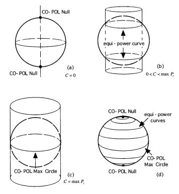
Fig. 5. Equi-power curves in the case of the co-pol channel when  $G_c^2(n) = -G_c^1(n)$ .
