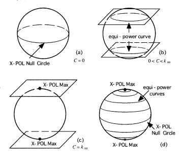
Fig. 6. Equi-power curves in the case of the cross-pol channel when  $G_c^2(n) = -G_c^1(n)$ .
