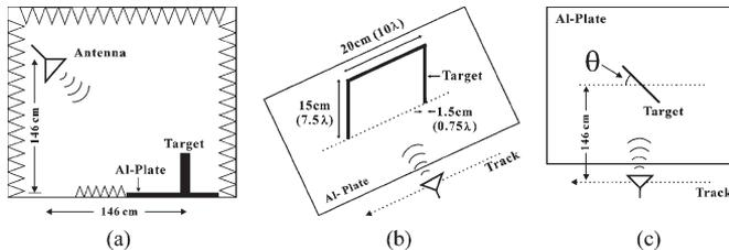
Fig. 3. Configuration of laboratory measurements. (a) Antenna and target geometry. (b) Target size. (c) Target orientation angle ( $\theta$ ), which is zero when the horizontal pole is oriented normal to the radar look direction.
