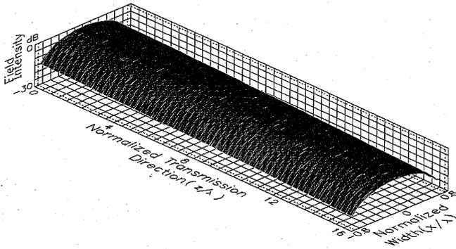
Fig. 4. Field pattern in hollow tunnel.
