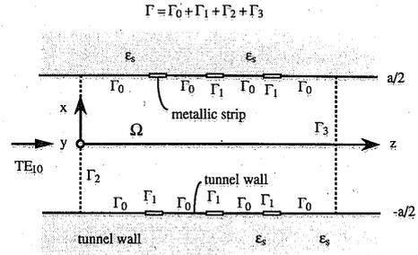
Fig. 2. Plane view of two-dimensional tunnel and the boundary  $\Gamma$ .
