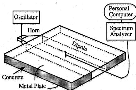
Fig. 10. Measurement scheme.
