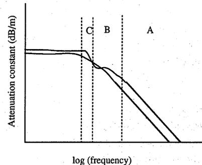
Fig. 1. Typical frequency characteristics of attenuation constants.
