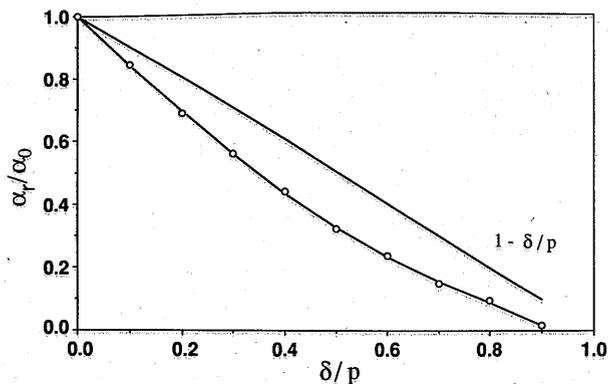
Fig. 9. Ratio of attenuation constant  $\alpha_s/\alpha_0$  as a function of  $\delta/p$ .
