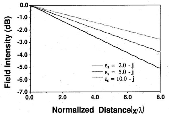
Fig. 6. Field strength as a function of normalized transmission distance along the center line of tunnel.
