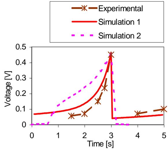
Fig. 6. An example of experimental result and numerical simulation from Run 6. Simulation 1: The magnetic flux density is spatially variable. Simulation 2: The magnetic flux density is uniformly 0.3 T.
