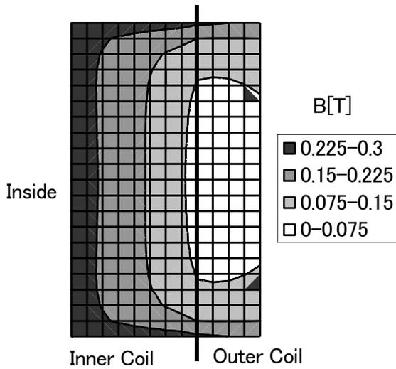
Fig. 7. Magnetic flux density distribution at 100 A.
