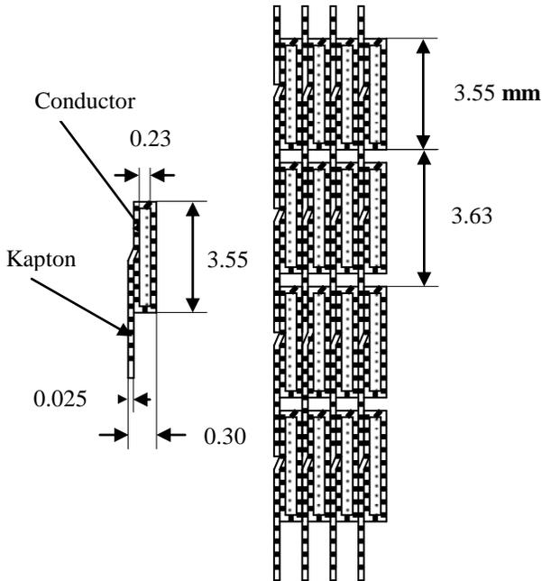
Fig. 4. Details showing conductor and insulator.
