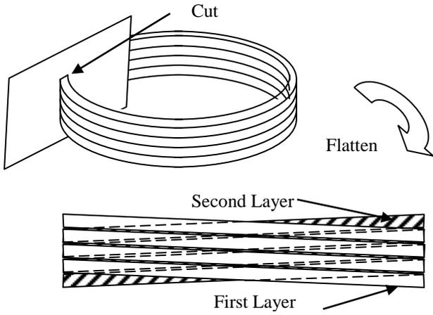
Fig. 3. Detail of two adjacent layers
