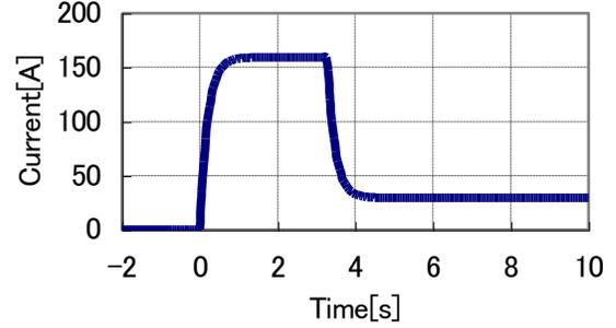
Fig. 2. An example of current waveform. A large pulse and operating current.
