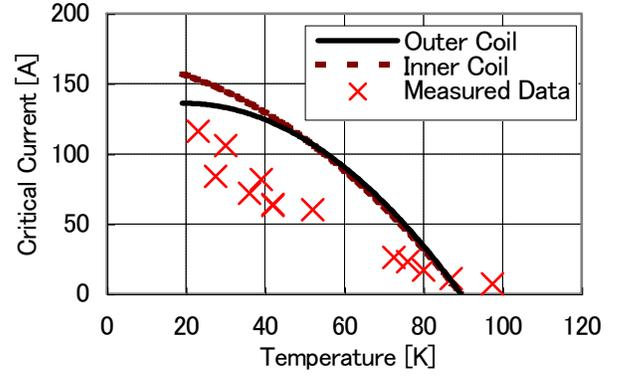
Fig. 5. Critical current curves estimated for the simulation and measured data (X).
