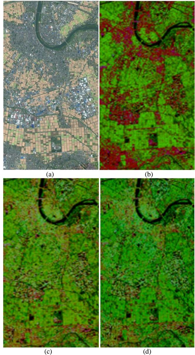
Fig. 2. Close-up areas of black box areas on Fig. 1, color-coded decomposition image with Red ( $m_d$ : double bounce), Green ( $m_v$ : volume scattering), Blue ( $m_s$ : surface scattering): (a) Google optical image (b) new hybrid decomposition with rotation about line of sight and extended volume scattering model (c) original hybrid decomposition with rotation about line of sight (d) original hybrid decomposition.
