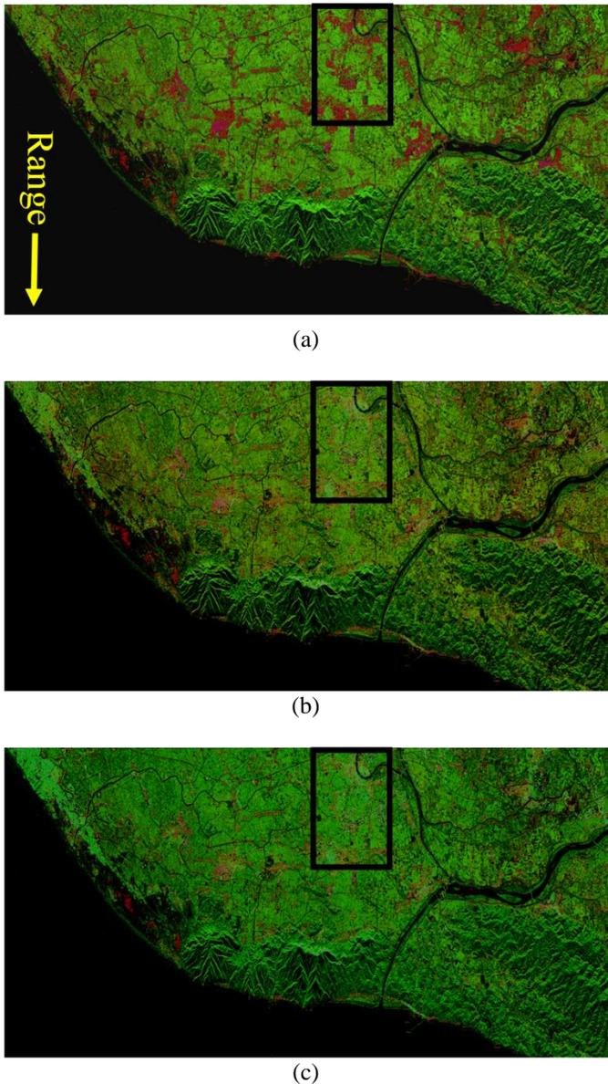
Fig. 1. Color-coded decomposition image with Red ( $m_d$ : double bounce), Green ( $m_v$ : volume scattering), Blue ( $m_s$ : surface scattering) (a) new hybrid decomposition with rotation about line of sight (real unitary transformation only) and extended volume scattering model (b) original hybrid decomposition with rotation about line of sight (real unitary transformation only) (c) original hybrid decomposition
