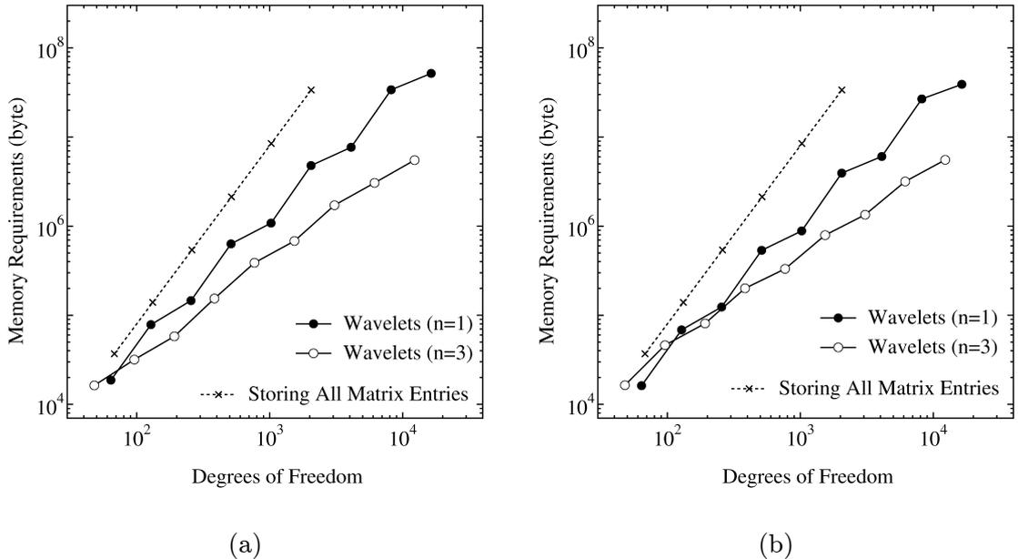
Figure 10: Memory requirements for matrix entries. Piecewise constant wavelets are used for the bases. (a) Ex.1. (b) Ex.2.
