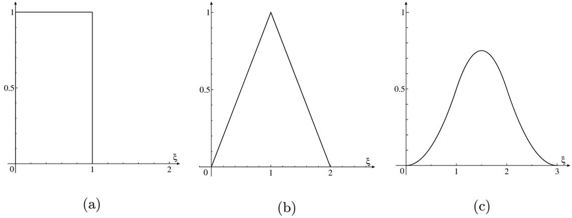
Figure 1: Examples of the scaling function. (a) Piecewise constant scaling function  $\phi^0(\xi)$ . (b) Piecewise linear scaling function  $\phi^1(\xi)$ . (c) Piecewise quadratic scaling function  $\phi^2(\xi)$ .
