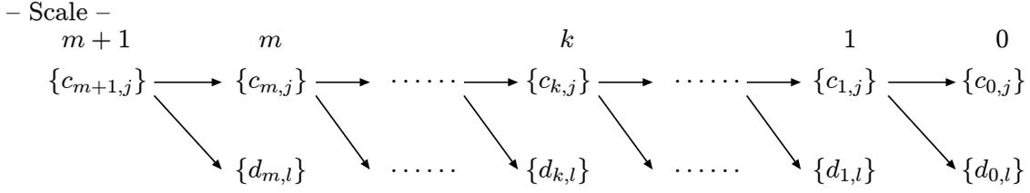
Figure 8: Fast wavelet transform. Expansion coefficients are evaluated in order as shown the arrows in this figure.
