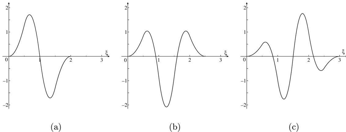
Figure 4: Piecewise quadratic non-orthogonal wavelets. (a) Wavelet  $\psi_1^2(\xi)$ . (b) Wavelet  $\psi_2^2(\xi)$ . (c) Wavelet  $\psi_3^2(\xi)$ .
