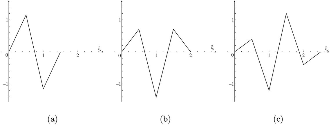
Figure 3: Piecewise linear non-orthogonal wavelets. (a) Wavelet  $\psi_1^1(\xi)$ . (b) Wavelet  $\psi_2^1(\xi)$ . (c) Wavelet  $\psi_3^1(\xi)$ .
