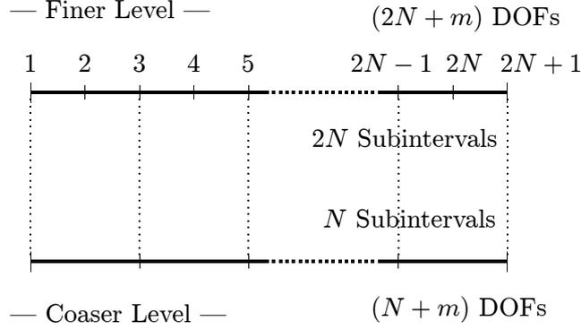
Figure 5: Finite interval under two-scale subdivision. The number of subintervals and DOFs are  $N$  and  $(N + m)$  for coarser scale,  $2N$  and  $(2N + m)$  for finer scale, respectively. In finer scale,  $(2N + 1)$  knots are required.
