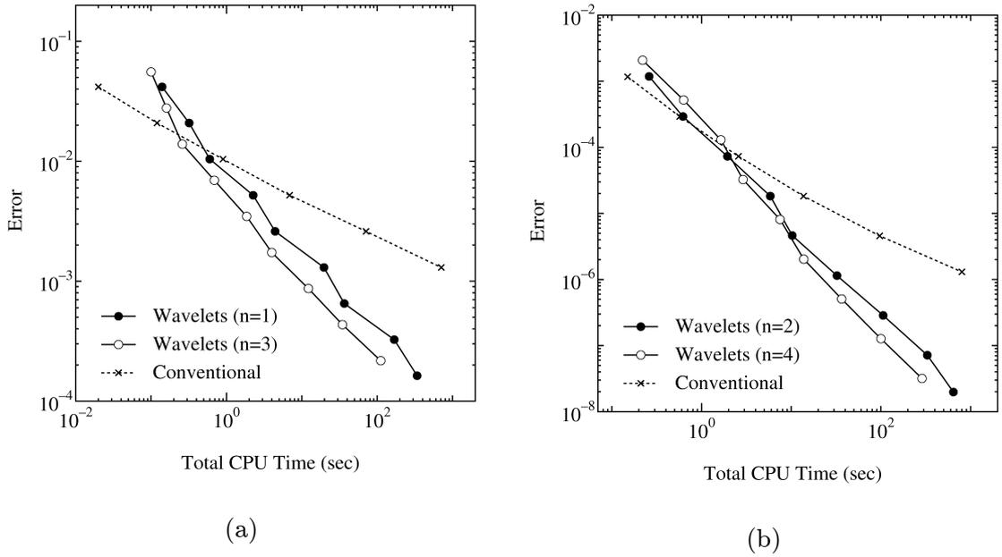
Figure 13: Relation between total CPU time and  $L^2$  norm of error in Ex.1. (a) Piecewise constant wavelets. (b) Piecewise linear wavelets.
