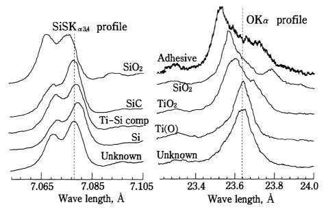
Fig. 7 Chemical bond states of Si and O on an abraded Ti surface. The profiles of Si satellite  $K_{\alpha_{3,4}}$  and O  $K_{\alpha}$  spectra of the contaminant were compared with those of standard substances. "Ti-Si comp" represents a net-shape and titanium silicide-like phase existing in the reaction zone of a titanium casting. "Ti(O)" is solute oxygen in the  $\alpha$ -case of a titanium casting.
