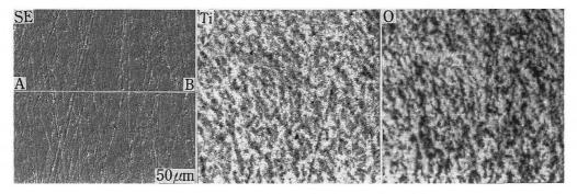
Fig. 2 Element distributions on an abraded Ti surface. Together with an 18-8 stainless steel chipping band, the specimen was resin-embedded and abraded to #1,000 grit.
