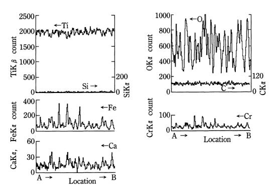
Fig. 3 Line analysis profiles of Ti, Si, O, C, Fe, Cr, and Ca along the line AB in the SE image of Fig. 2
