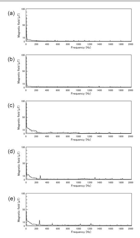
Fig. 3 Low frequency magnetic fields produced by electric toothbrushes.
