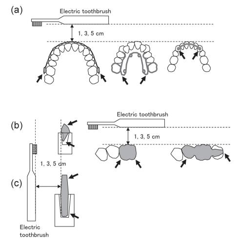
Fig. 1 Schematic representation of experiments for estimating induced electric currents.
