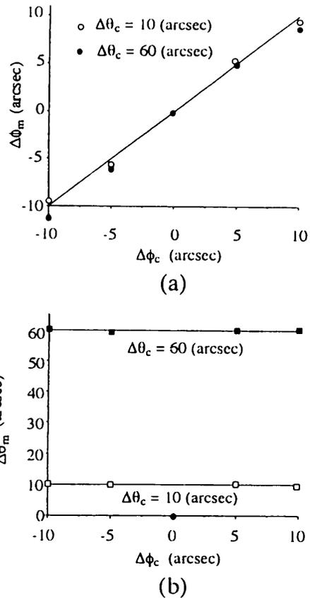
Fig. 7. Measurement results of errors  $E_{\Delta\phi}$  and  $E_{\Delta\theta}$  at  $\Delta\theta_c = 10$  and  $60$  arcsec, respectively.
