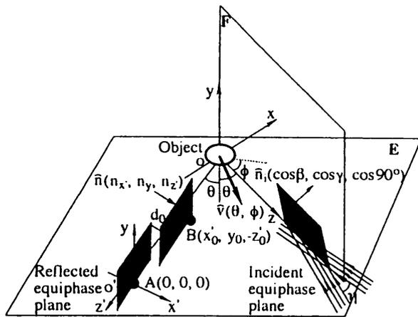
Fig. 1. Reflection of a parallel interference pattern.
