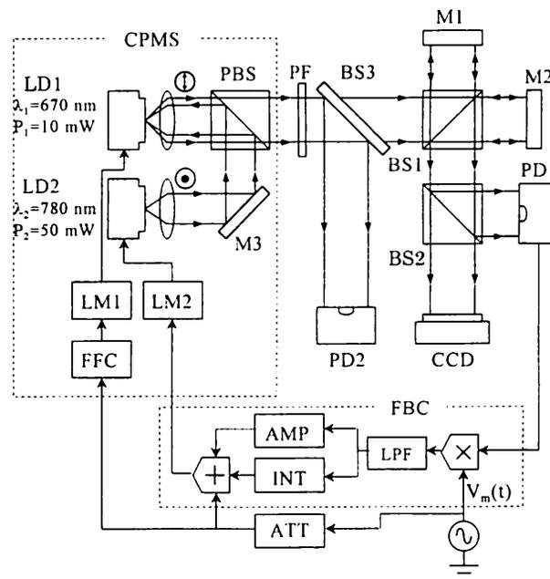
Fig. 4. Experimental setup of the  $CP$ -modulating system with a feedback control. CPMS, current and photothermal modulating system; FBC, feedback controller; LD1, laser for a light source; LD2, heating laser; PBS, polarizing beam splitter; BS, beam splitter; M, mirror; AMP, amplifier; INT, integrator; ATT, attenuator.
