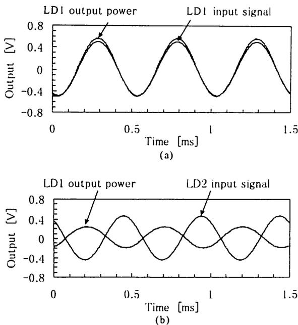
Fig. 5. Optical power changes in the LD with respect to the injection current (a) for LD1 and (b) for LD2.
