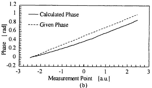
Fig. 10. Deviations of the phase extracted from the intensity-modulated interference signal with visibility of 100%.  $\gamma$ , the coefficient of the optical power changes, are (a) 0.1 and (b) 0.5.
