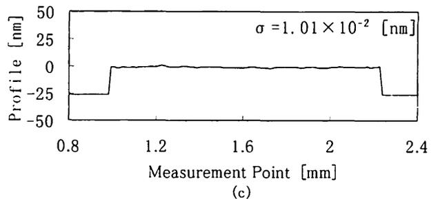
Fig. 13. Surface profile of flat mirror measured with (a)  $C$  modulation, (b)  $P$  modulation, and (c)  $CP$  modulation.  $\sigma$ 's are the differences between the fitting line and the fitting curve, and they indicate that  $CP$  modulation is useful for reducing the deviation caused by the intensity modulation.
