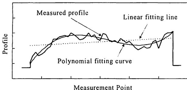
Fig. 12. Schematic of calculation method for  $\sigma$ , which is denoted by the rms value of the difference between the linear fitting line and the polynomial fitting curve of degree three.
