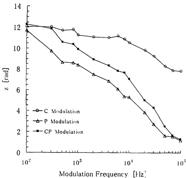
Fig. 8. Dependency of modulation depth  $z$  on modulation frequency.
