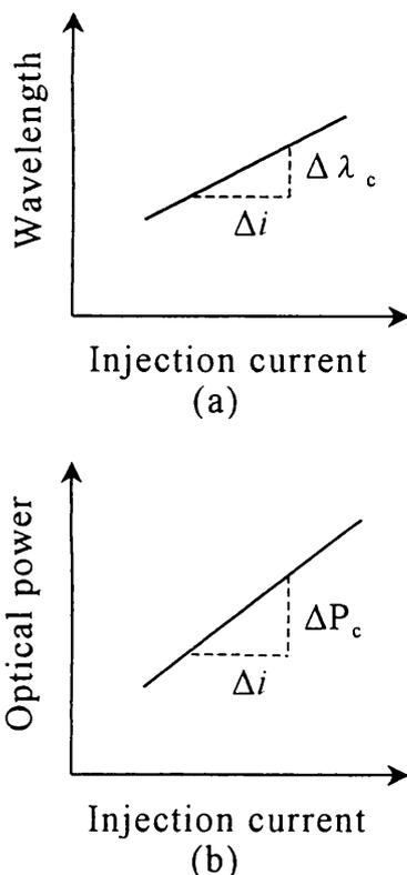
Fig. 2. Characteristics of LD's (a) wavelength tunability and (b) optical power change with injection current.
