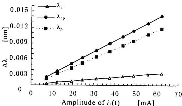
Fig. 9. Wavelength shift corresponding to amplitude of  $i_2(t)$ . In the  $CP$  modulation, wavelength shifts by  $\lambda_p$  and  $\lambda_c$  with the  $P$  modulation and the  $C$  modulation, respectively. Total wavelength shift  $\lambda_{cp}$  becomes the sum of  $\lambda_p$  and  $\lambda_c$  in  $CP$  modulation.
