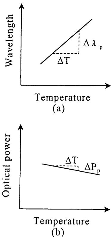
Fig. 3. Characteristics of LD's (a) wavelength tunability and (b) optical power change with temperature.  $\Delta P_p/\Delta T$  is negative.
