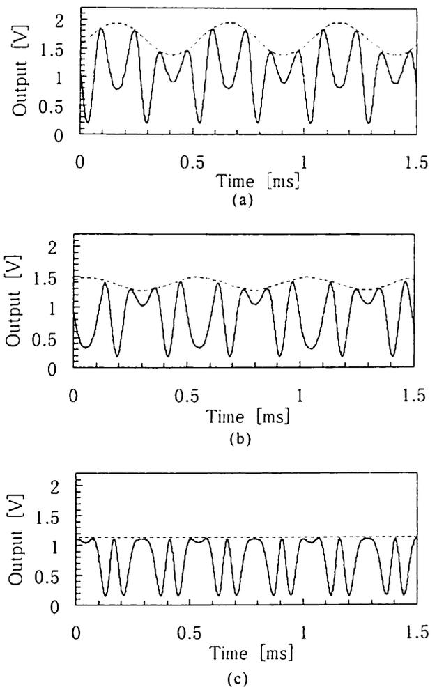
Fig. 7. Interference signals obtained by (a) *C* modulation, (b) *P* modulation, and (c) *CP* modulation. Modulation frequency is 2 kHz. Dashed curve, distortion introduced by the intensity modulation.
