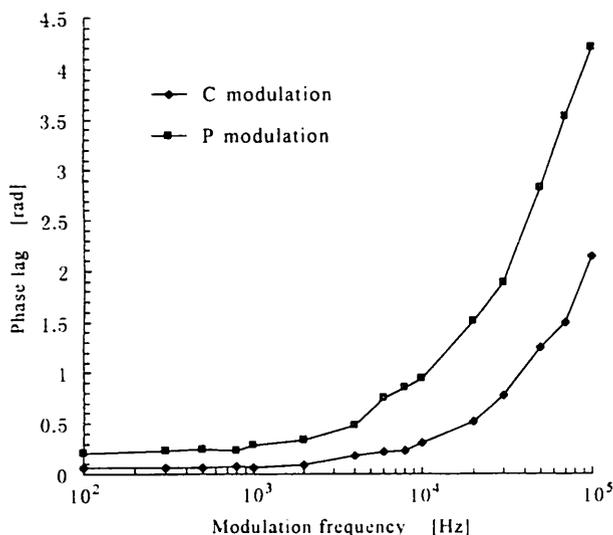
Fig. 6. Phase lags in the *C*- and the *P*-modulated interference signals with respect to the frequency of the injection current.
