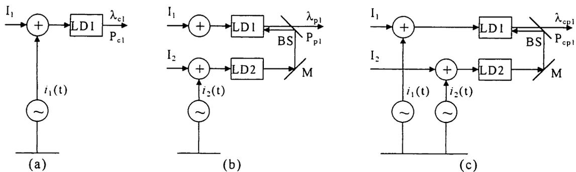
Fig. 1. Schematic of (a) *C* modulation, (b) *P* modulation, and (c) *CP* modulation. BS, beam splitter; *I*, dc bias current; LD1, laser for a light source; LD2, heating laser; M, mirror.
