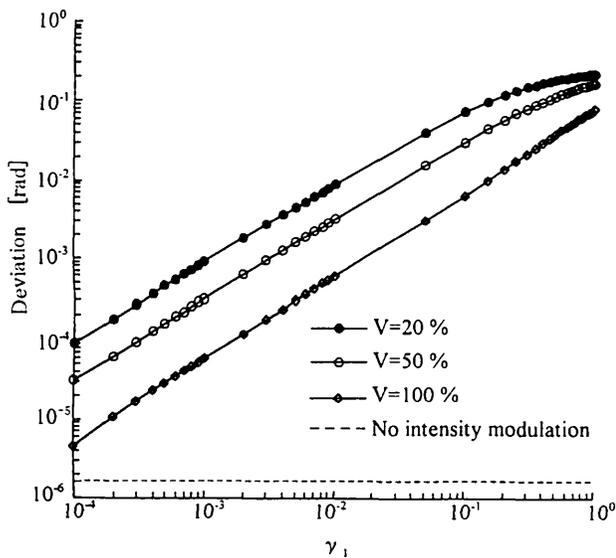
Fig. 11. Dependency of deviations on coefficient  $\gamma_1$ . Although the deviation reduces as the visibility increases, considerable error still remains.
