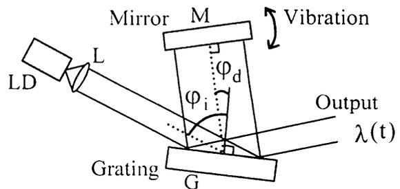
Fig. 2. Configuration of the SWS TLD.
