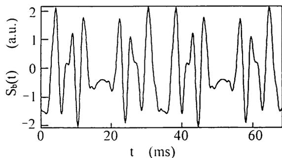
Fig. 3. Objective signal  $S_b(t)$  extracted from the interference signal detected for a vinyl sheet with two surfaces.
