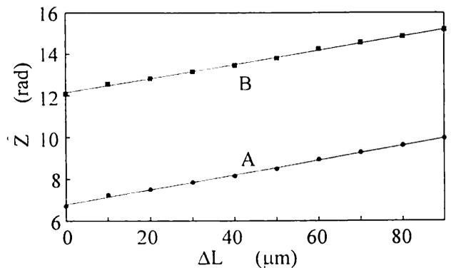
Fig. 8. Values of  $Z$  for the two surfaces, A and B, measured every time the object was displaced such that the change  $\Delta L$  in the OPD increased by  $10 \mu\text{m}$ .
