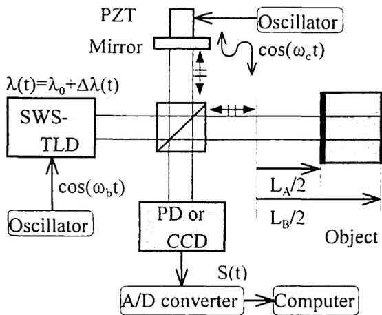
Fig. 1. Sinusoidal wavelength-scanning interferometric reflectometer: PZT, piezoelectric transducer; PD, photodiode; A/D, analog-to-digital.
