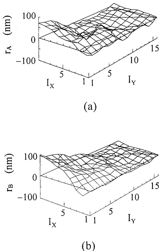
Fig. 14. Measured profiles of (a) the front surface and (b) the rear surface of the silica glass plate.
