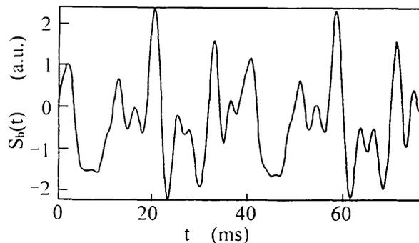
Fig. 12. Objective signal  $S_b(t)$  extracted from the interference signal detected for a silica glass plate with thickness of  $20 \mu\text{m}$ .
