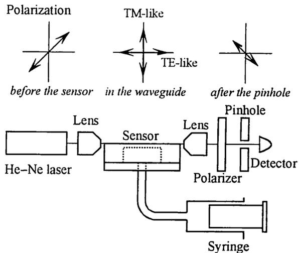
Fig. 4. Experimental setup to measure the output intensity as a function of the applied pressure.
