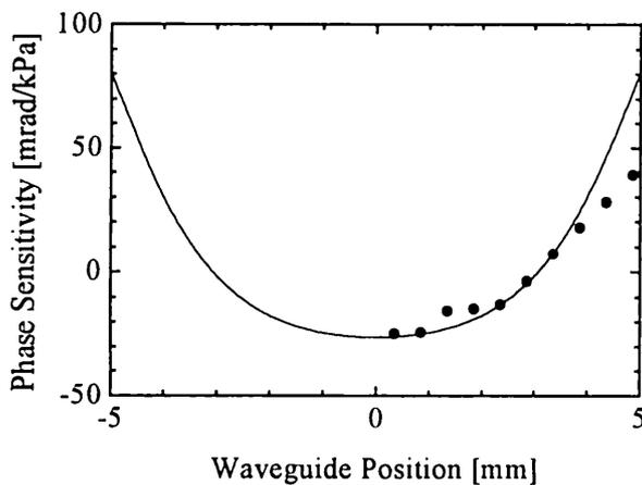
Fig. 6. Measured phase sensitivity as a function of the waveguide position on the diaphragm.
