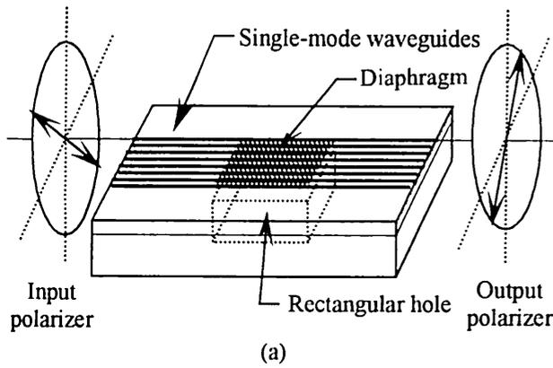
Fig. 1. (a) Schematic drawing of the integrated optic pressure sensor placed between a pair of crossed polarizers and (b) its cross sectional view. The sensor has 24 waveguides on the diaphragm to determine the relationship between phase sensitivity and waveguide position.
