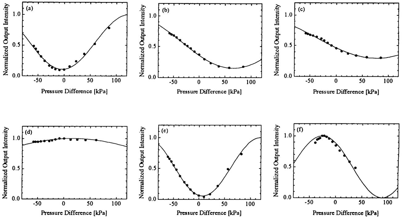
Fig. 5. These figures indicate the experimental results of normalized output intensity versus applied pressure difference for waveguides placed at (a) 0.35, (b) 1.35, (c) 2.35, (d) 3.35, and (e) 4.35 mm from the center of the diaphragm. Also, (f) is for a waveguide located 0.35 mm outside of the diaphragm edge.
