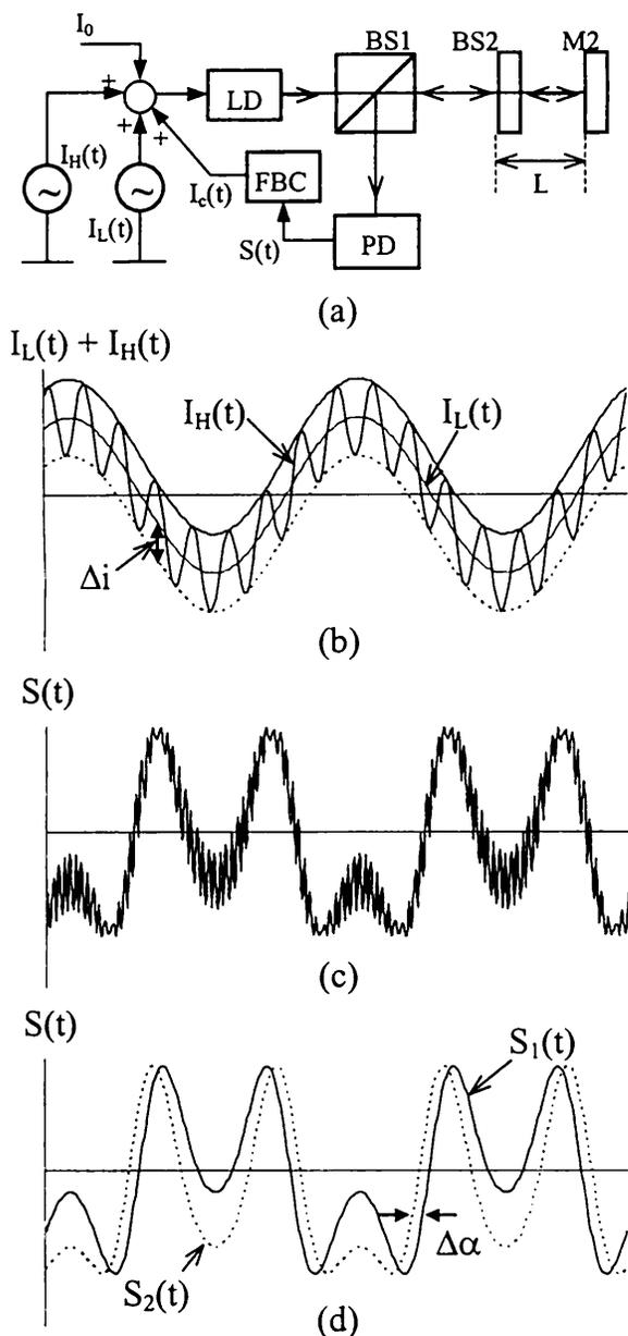
Fig. 1. Schematic of the DSPM technique and QTWI. (a) Basic architecture of the system: BS1, BS2, beam splitters; M2, mirror; FBC, feedback controller; PD, photodetector. (b) Modulating current for the DSPM technique, (c) DSPM interference signal, (d) separated interference signals for the QTWI.
