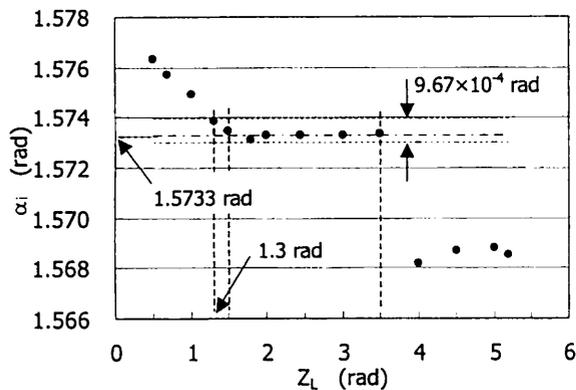
Fig. 7. Numerical calculation of phase detection with respect to  $Z_L$  in SPM interferometry.
