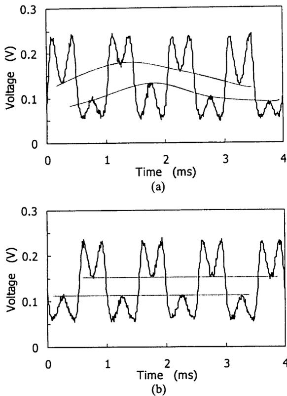
Fig. 6. Interference signals observed when the feedback control is (a) off and (b) on. Dotted curves indicate the phase deviation caused by the external disturbance.
