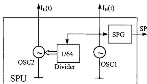
Fig. 4. Block diagram of the signal-processing unit: OSC1, OSC2, oscillators; SPG, sampling pulse generator; SP, sampling pulse; SPU, signal-processing unit.
