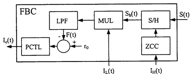
Fig. 2. Block diagram of the feedback controller: S/H, sample-and-hold circuit; ZCC, zero-cross circuit; MUL, multiplier; LPF, low-pass filter; PCTL, proportional controller; FBC, feedback controller.
