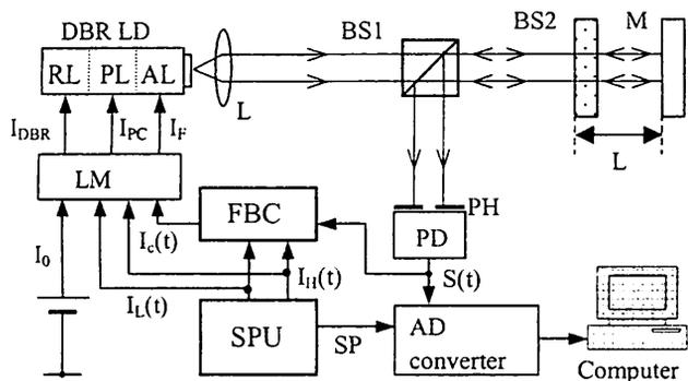
Fig. 3. Experimental setup: L's, lenses; BS1, BS2, beam splitters; M, mirror; FBC, feedback controller; PH, pinhole; PD, photodetector; SPU, signal-processing unit; LM, laser-diode modulator; RL, reflection-tuning layer; PL, phase-tuning layer; AL, active layer; AD, analog to digital.
