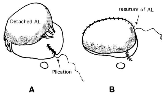
**Fig. 2.** Repair by modified Carpentier's method. **(A)** The anterior leaflet is detached from the annulus. The atrialized right ventricle is plicated longitudinally. **(B)** The detached anterior leaflet is sutured to the original annulus.
