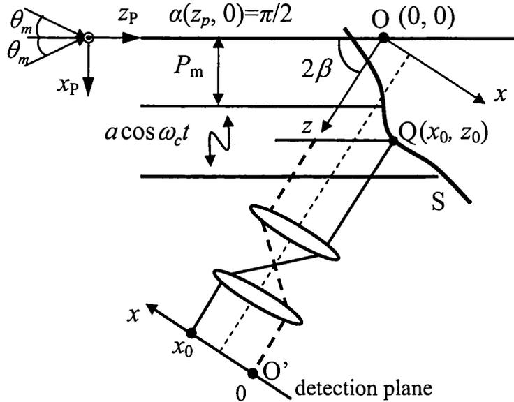
Fig.1 Schematic configuration for multiperiod fringe projection interferometer with sinusoidal phase-modulation.
