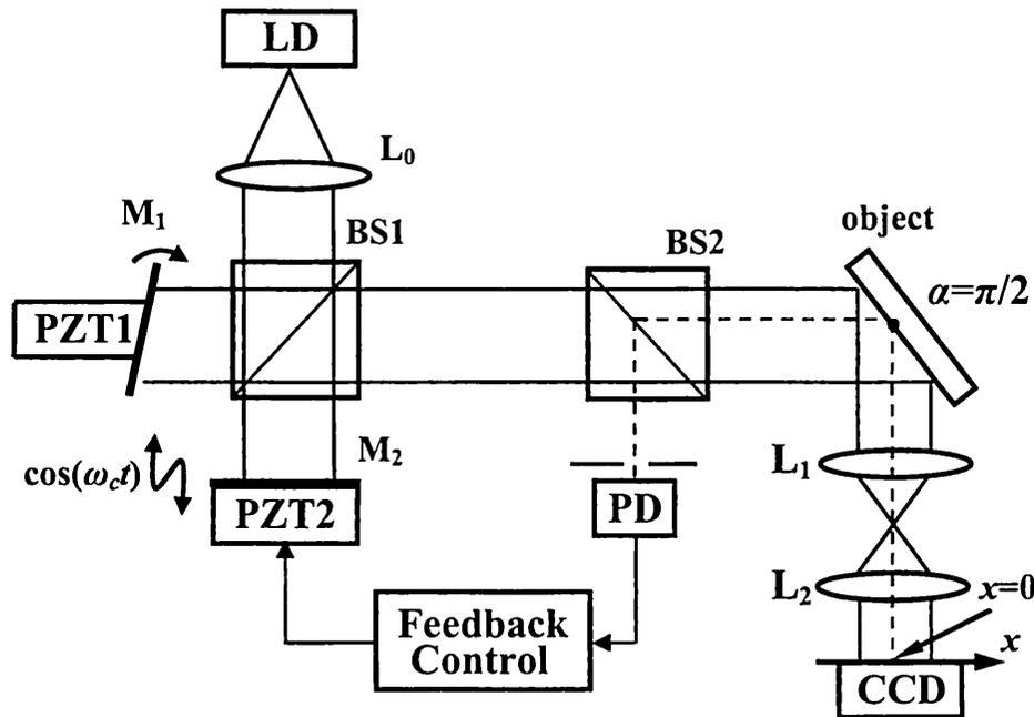
Fig. 3 Experiment setup of the multiperiod fringe projection interferometer.
