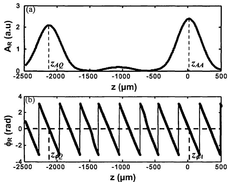
Fig. 4 Results of the back-propagation for one point of  $x_A = 2.90\text{mm}$  on the front surface and  $x_B = 3.30\text{mm}$  on the back surface of glass plate: (a) amplitude distribution  $A_R$ , (b) phase distribution  $\phi_R$ .
