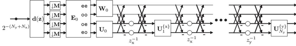
Fig. 2. Lattice structure of a 2-D non-separable GenLOT (forward transform).
