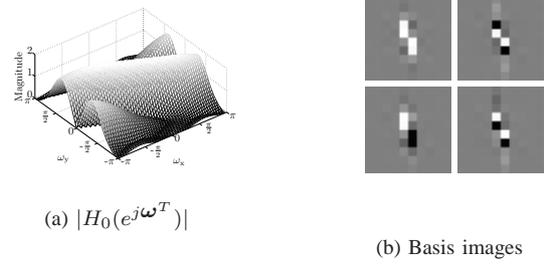
Fig. 3. A design example with the two-order TVMs of  $\phi = \cot^{-1} \alpha = \cot^{-1}(-2.0) \sim -0.4636[\text{rad}]$ , where  $[N_y, N_x]^T = [4, 4]^T$ , i.e. the basis images are of size  $10 \times 10$ .
