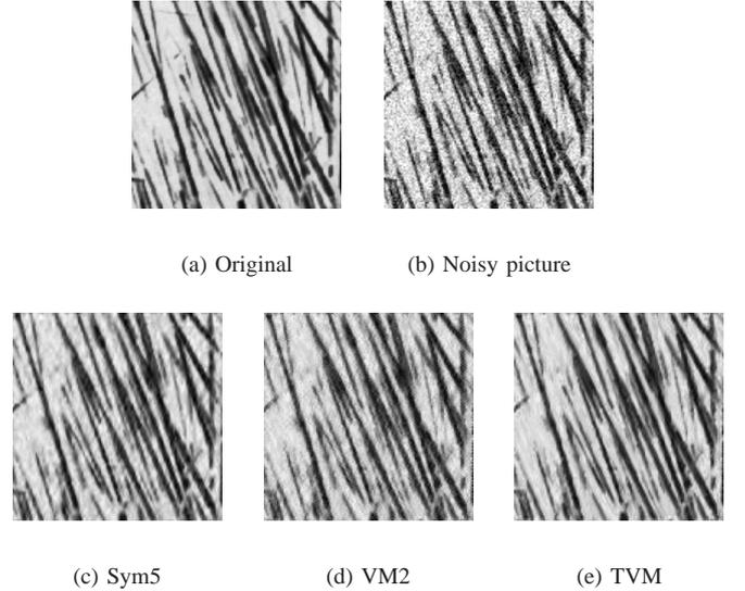
Fig. 4. Denoising results, for an 8-bit grayscale picture of size  $128 \times 128$  pixels. (a)Original picture, (b)Noisy picture with white Gaussian ( $\sigma = 30$ ). (c),(d) and (e) are denoised results, where Sym5, VM2 and TVM denote Symlets of index 5, DirLOT with the classical VM of order two and DirLOT with the two-order TVMs, respectively. The number of hierarchical levels is three.
