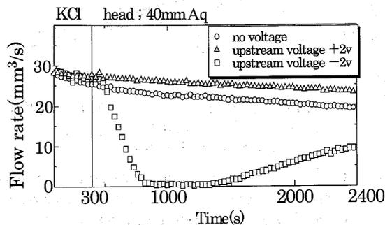
Fig. 7 Flow rate as a function of time for KCl solution in water. The experimental condition is the same as in Fig. 6.
