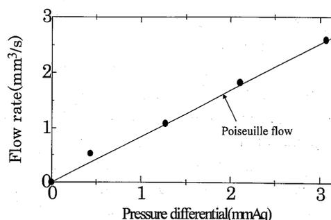
Fig. 12 Flow rate against pressure differential between upstream and downstream positions of the membrane. Solid line indicates the theoretical line obtained assuming Poiseuille flow in the pore. Head is 0 mmAq.
