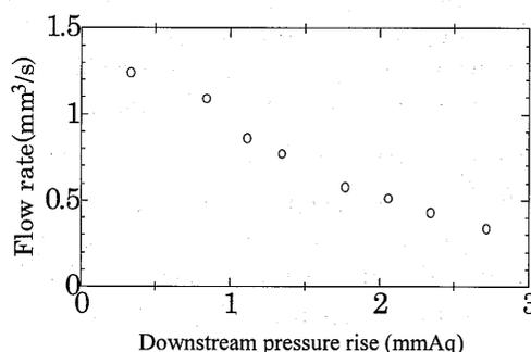
Fig. 13 Flow rate against the pressure applied at the downstream position. This corresponds to the pump performance.
