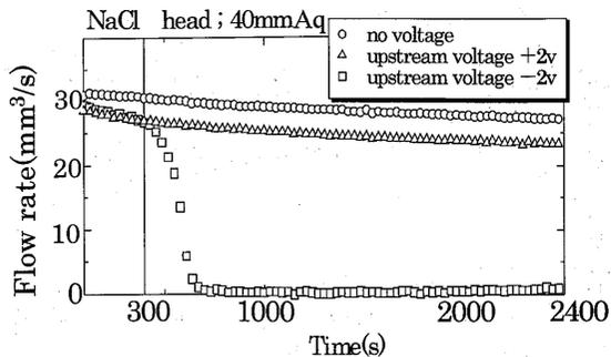
Fig. 6 Flow rate as a function of time for NaCl solution in water. Electric poles are a silver plate as plus pole and a zinc plate as minus pole. Nickel membrane is used and the diameter of the pore is  $5.01 \mu\text{m}$ . Head is  $40 \text{ mm Aq}$ .
