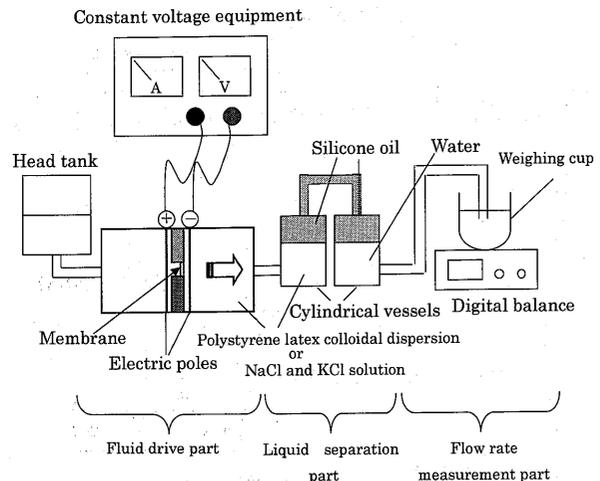
Fig. 8 Fabrication for the experiment of micropump
