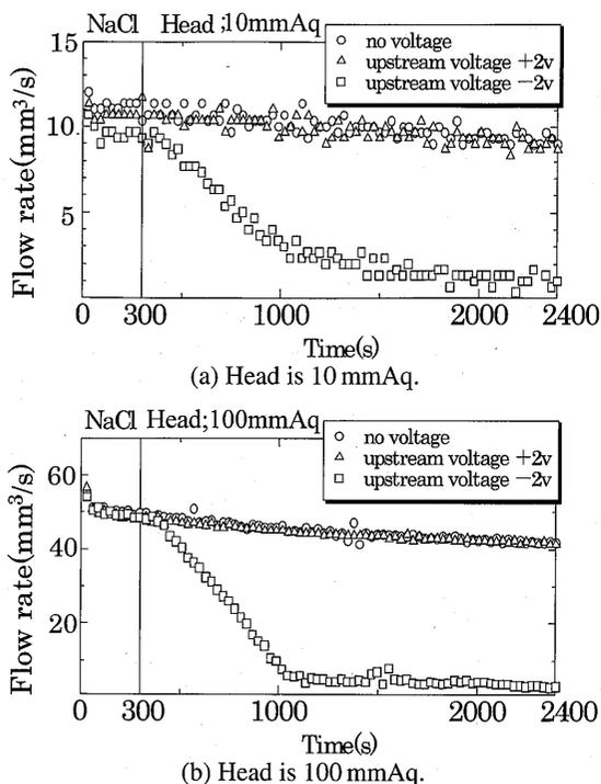
Fig. 3 Flow rate as a function of time for NaCl solution in water. The experimental condition is the same as in Fig. 2.
