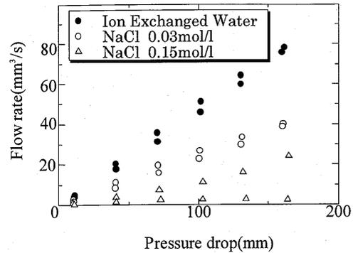
Fig. 14 Flow rate against pressure drop in the case that solutions are made to flow by heads with no voltage. Polycarbonate membrane is used and the diameter of the pore is  $1.2 \mu\text{m}$ . The flow rate is seen to decrease as the concentration of NaCl increases.
