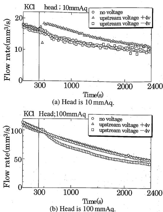
Fig. 4 Flow rate as a function of time for KCl solution in water. Electric poles are stainless plates. Nickel membrane is used and the diameter of the pore is 5.83  $\mu\text{m}$ .
