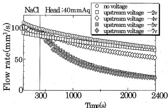
Fig. 5 Flow rate as a function of time for NaCl solution in water. Electric poles are stainless plates. Polycarbonate membrane is used and the diameter of the pore is 5.0  $\mu\text{m}$ . Head is 40 mmAq.
